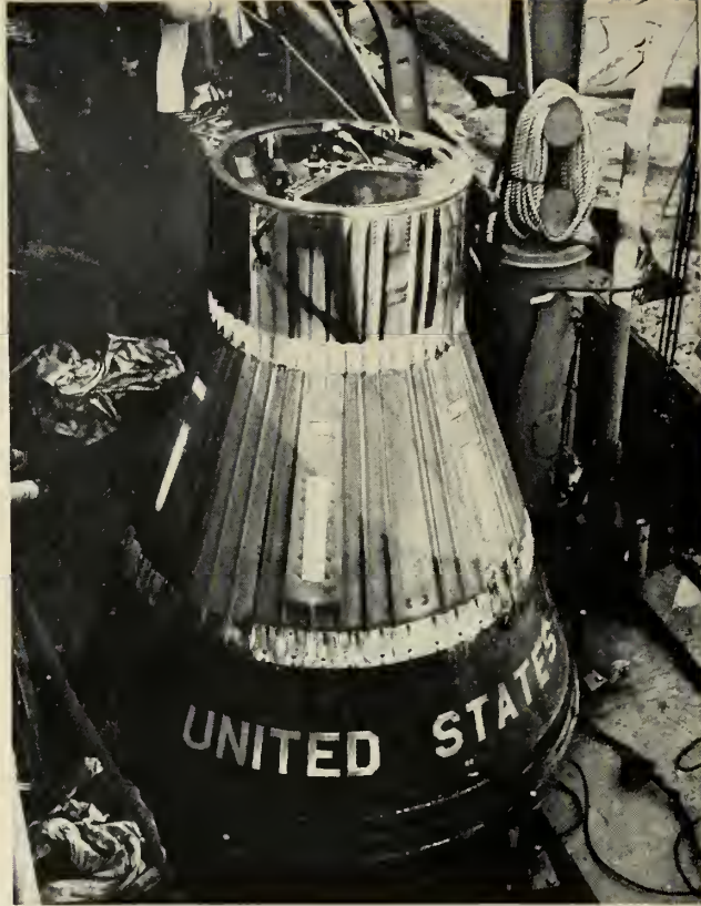
THE ATLAS MISSILE LAUNCHED NASA'S one-ton instrumented capsule similar to the one that will carry a man into space orbit. Initial landing phase began at 45,000 feet when a barometric switch fired a charge which deployed a Radioplane stabilization parachute directly aft into the airstream. At the same time, radar chaff was ejected to scatter into a 600-square-foot pattern to provide for radar locating and tracking.
