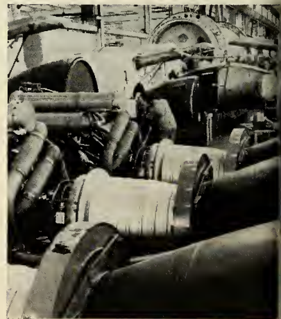
ENGINE sections, tanks, and guidance and control sections are joined and all cables and lines attached to Thor .
