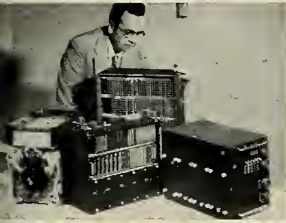
The completely transistorized RW-300 airborne digital computer has a volume of 4.19 cu. ft. and weighs only 203 lbs., including power supply
