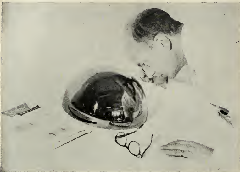
LARGEST INFRARED dome manufactured in one piece, which will be used on classified IR search equipment has been delivered to NADC, Johnsville.
