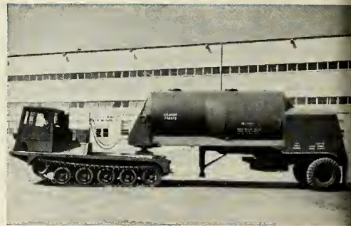
As a multi-service prime mover, the FMC-built ABMA Tractor is powered for moving heaviest loads on short or long hauls with ease and dispatch. This sure-footed, tracked vehicle handles all types of trailers, is equally capable on soft, rough or surfaced ground.
