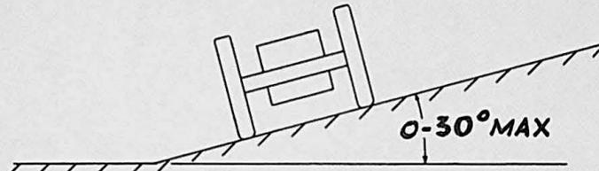
1. TRAVERSING THE SIDE OF A SLOPE
