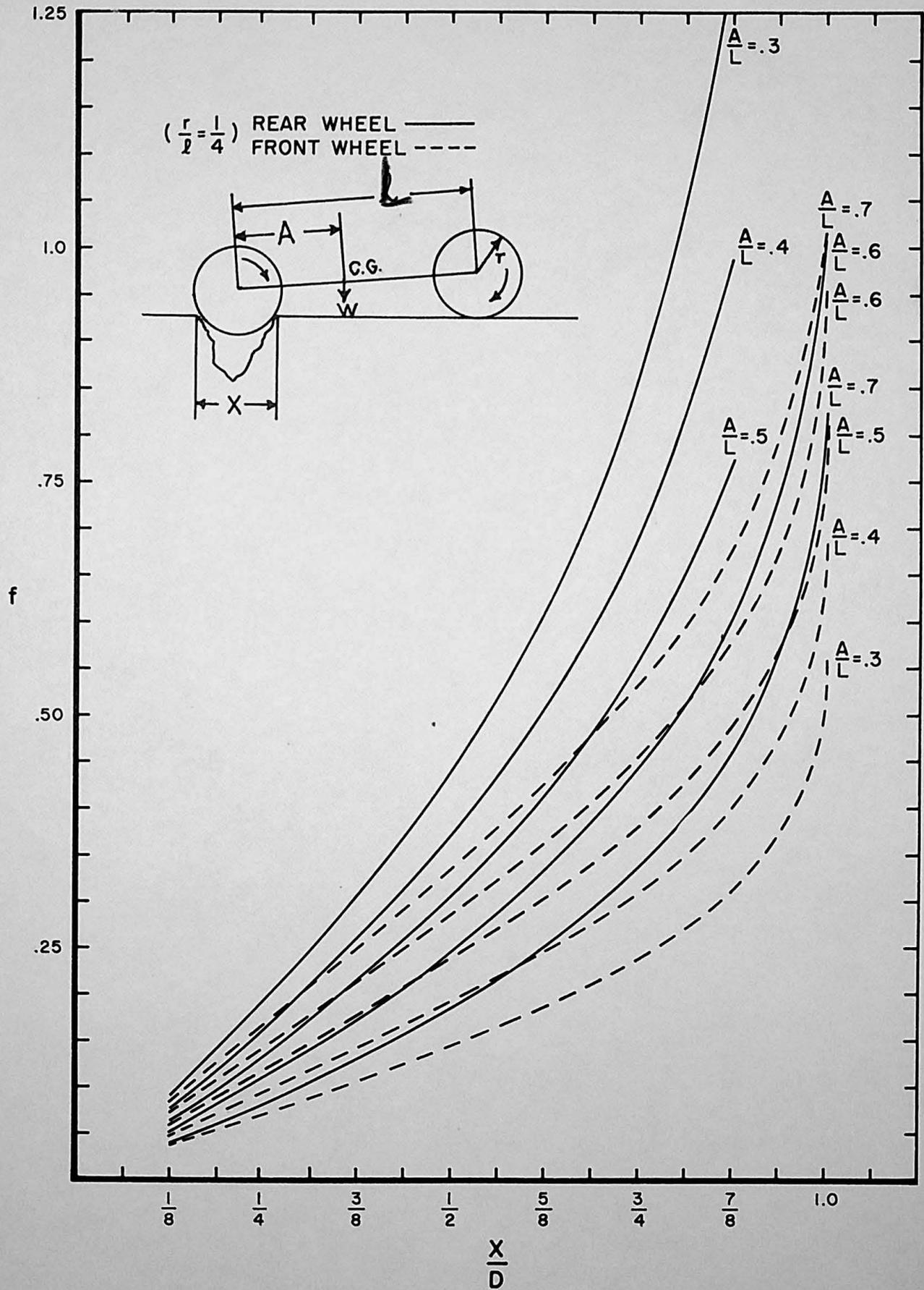
FRICITION REQUIREMENTS FOR FOUR WHEEL DRIVE VEHICLE NEGOTIATING A CREVICE.
