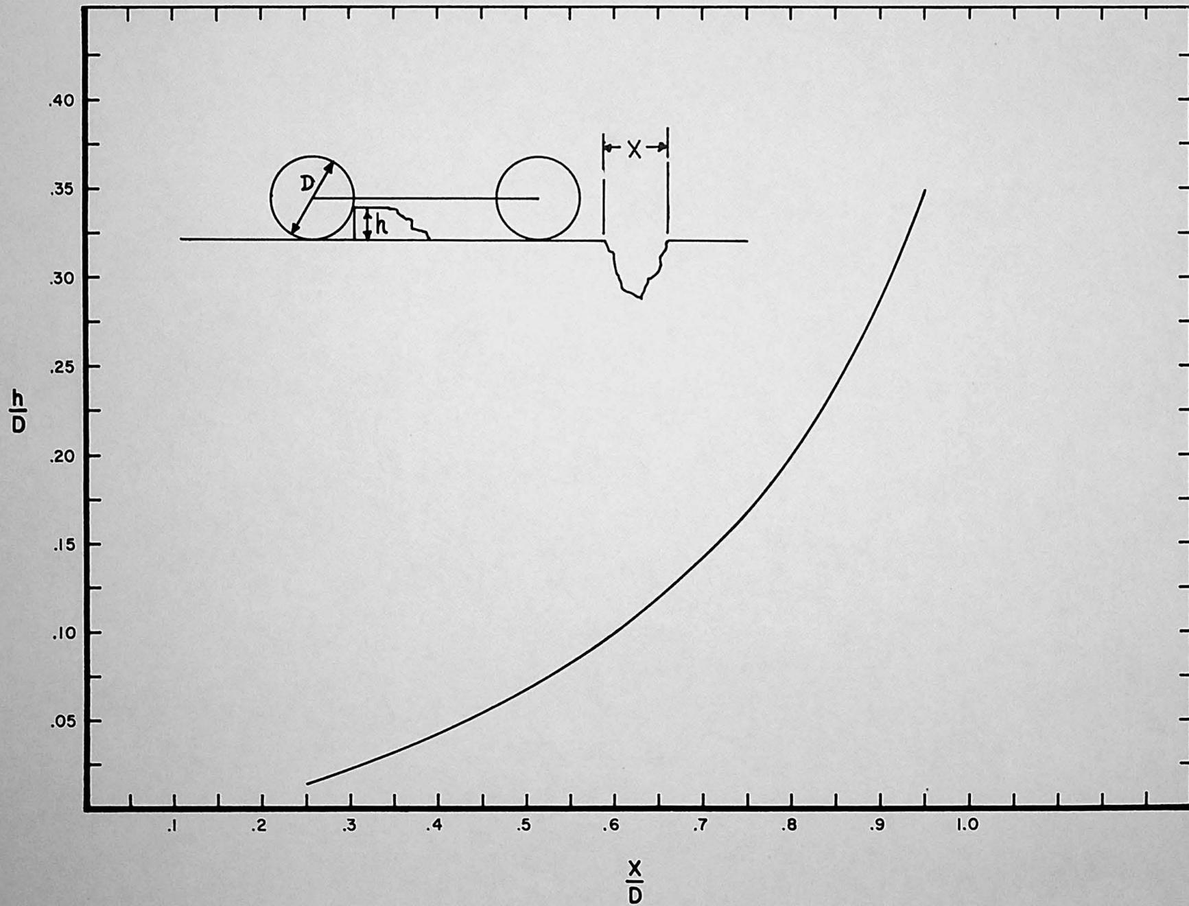
CREVICE WIDTH CONVERTED TO OBSTACLE HEIGHT OF EQUAL NEGOTIABILITY
