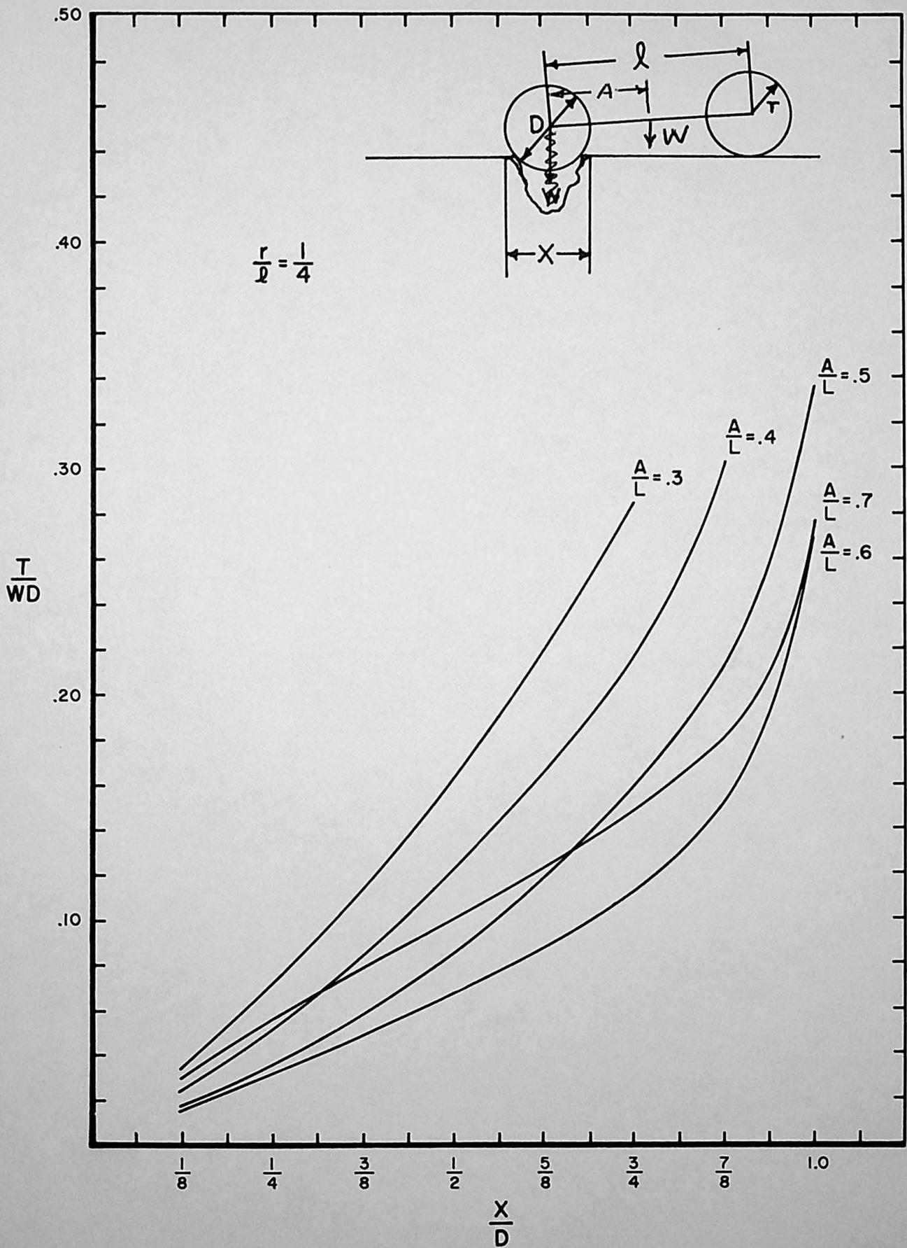
MAXIMUM AXLE TORQUE REQUIREMENTS FOR FOUR WHEEL DRIVE VEHICLE NEGOTIATING A CREVICE.
