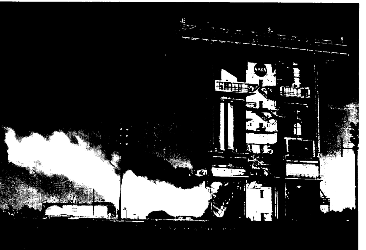
STATIC TEST —The first Saturn S-IB booster, built by Chrysler Space Division at Michoud Assembly Facility in New Orleans, is successfully static test fired at Marshall Space Flight Center in Huntsville, Ala.
