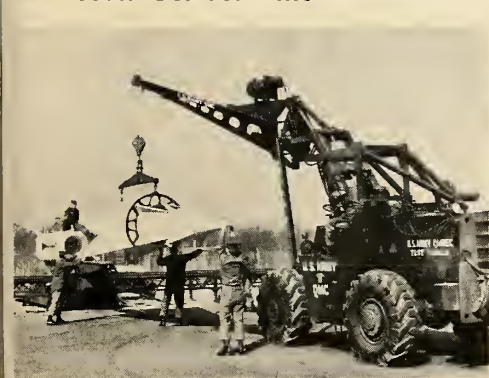
QUARTERMASTER Corps' "Ranger," all-purpose vehicle is being used to lift Nike-Hercules to its launching rack for union with the booster. It can pull 19,000 lbs. and lift 10,000 lbs.
