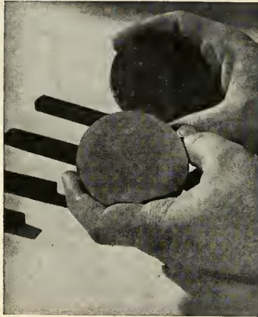
HEAT- and oxidation-resistant coating is visible on the lower test disc. Upper disc has not been exposed to high temperatures.
