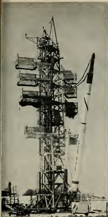
SCOUT STANDS at launch tower, ready for launching at 85° angle of elevation.
