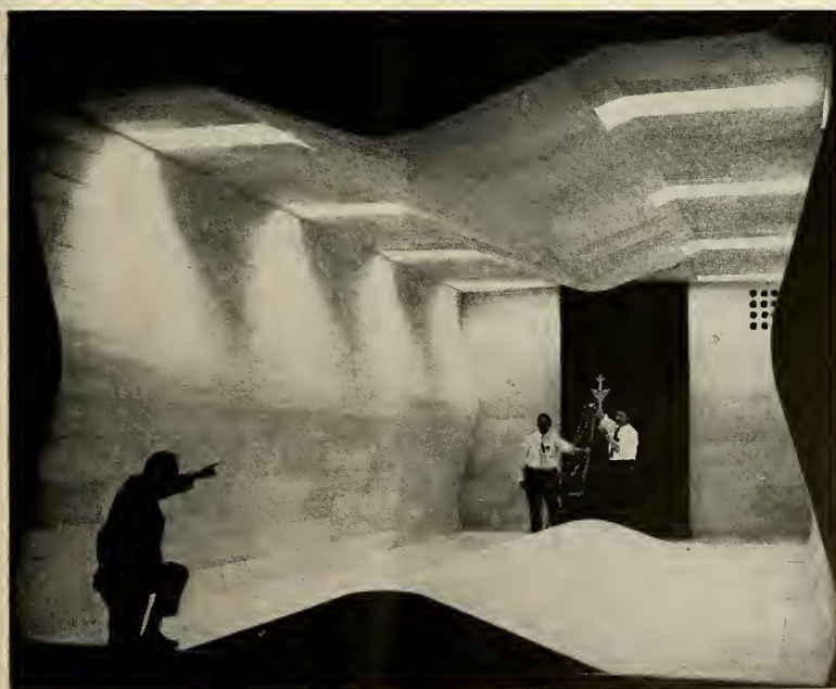
BULGES AND BUCKLES with a purpose were built into this room at Republic Aviation's new Farmingdale, N.Y., Research and Development Center. Gibson-Girl build of walls makes almost completely echo-free environment for testing antennas.
