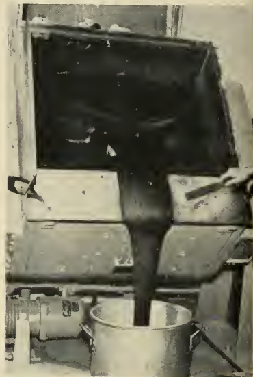
POURING polyvinyl chloride-based propellant at Atlantic Research Corp.
