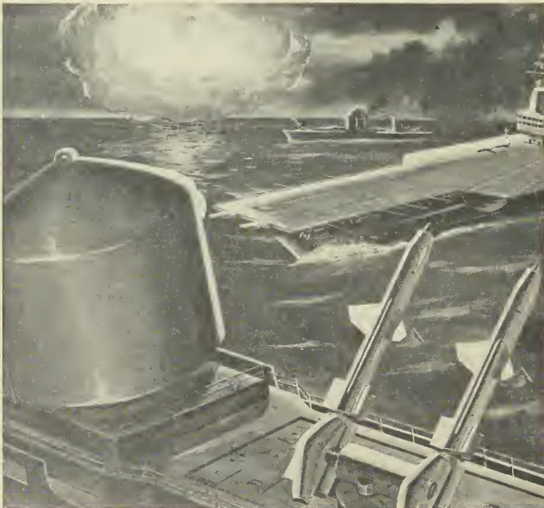
ARTIST'S CONCEPTION of Typhon in action. Missile cruiser is shown with dome of new type of radar antenna which can keep track of several missiles at one time.
