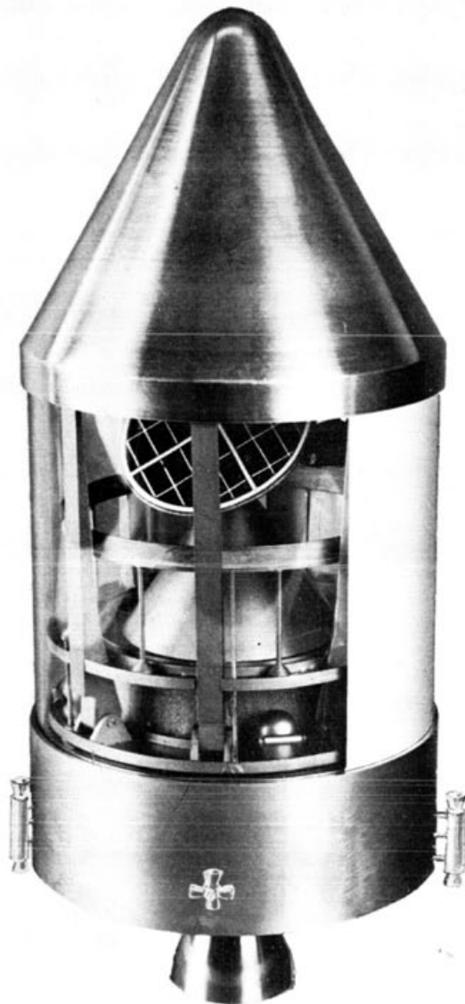
FIG. I.2 LUNAR LANDING VEHICLE FOR STATIONARY PACKET
