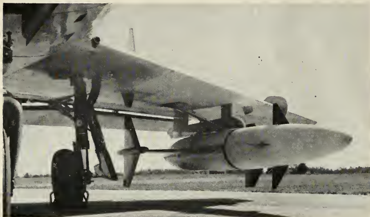
SWEDISH Type 304 air-to-surface missile mounted under aircraft wing.
