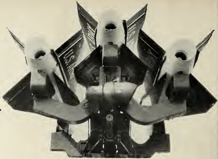
This unusual rear-view shot of Raytheon's Hawks shows details of tri-mount launcher.
