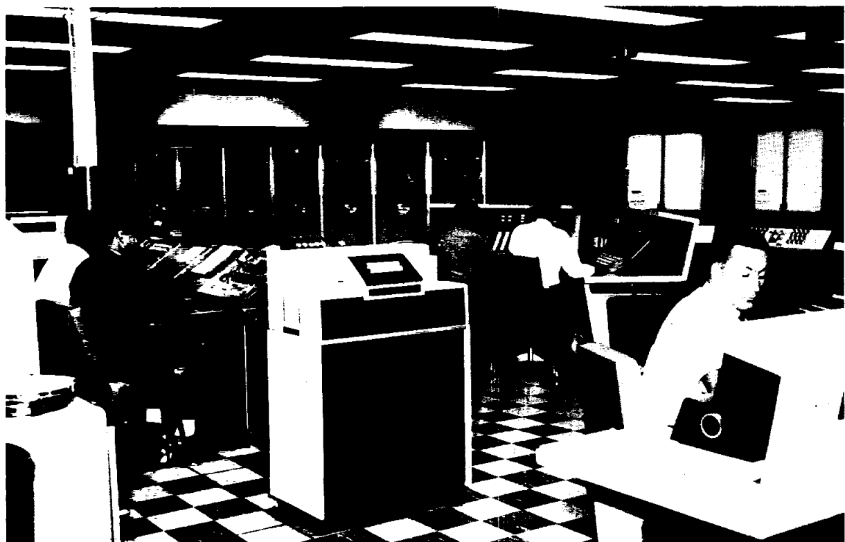
NERVE CENTER OF EMTR—This is the "nerve" center of the Eastern Missile Tracking Range, Cape Kennedy, with two Control Data 3600 computers in the real-time computer system. Besides tracking the missile, the system gives the range safety officer a continuous impact prediction, enabling him to make a go-or-destroy decision.
