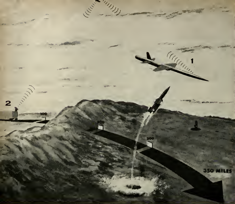
SPERRY MICROWAVE command system: missile target (1) is controlled by airborne director (3), which relays the microwave signals from ground director station (2).
