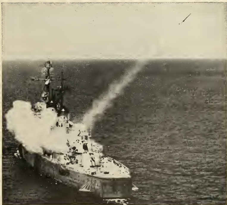
USS NORFOLK FIRES deadly ASROC during evaluation tests off Key West. The now-operational missile is unofficially estimated to be effective up to eight miles.
