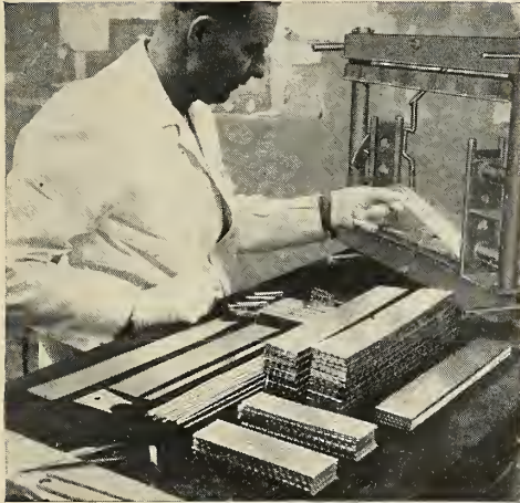
UAP worker assembles multiple parts in fixture for heat exchanger care. Gloves guard against contamination of aluminum prior to brazing.
