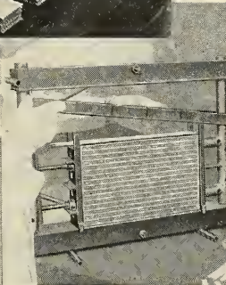
Fixturing is complete. Assembly proceeds rapidly since banding of parts is achieved in a single dip-brazing operation.
