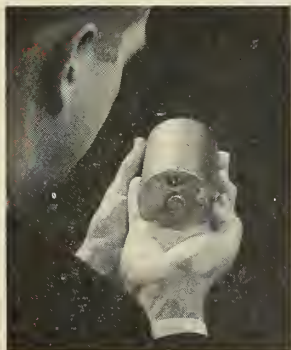
New small free gyro, "inner ear" of the simplified inertial platform.
