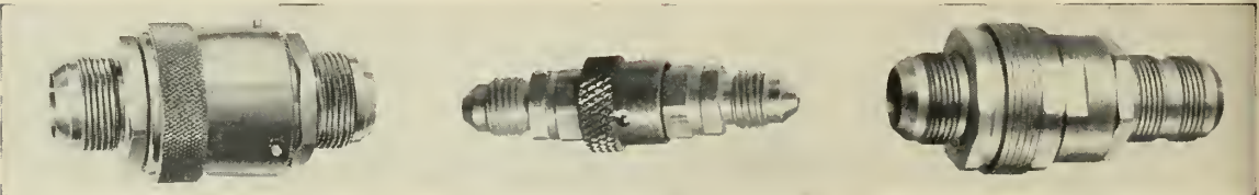
3750 Series Quick Disconnect Coupling for ¼" to 1½" lines features visual lock indicator pins for foolproof connection. Full flow design with low pressure drop.
