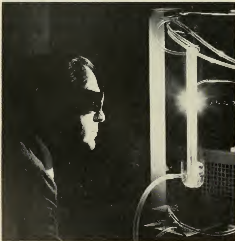
ZONE MELTING applied to a rod of powdered boron. A method for coating boron powder with boric acid made it possible for Bell Laboratories to process strong, pressed forms of boron.
