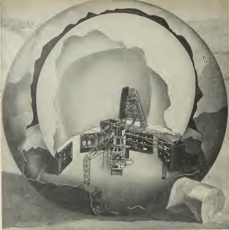
CUTAWAY DRAWING of TPS-27 shows painted-on antenna (gray area in center) in inflated Paraballoon. Entire system is enclosed in pressure-inflated radome approximately 50 feet in diameter.
