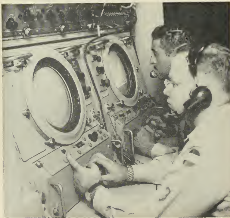
FRESCANAR scope on left displays target range and bearing, that on right, altitude. Data is instantaneously transmitted to missile antiaircraft batteries which automatically track targets. Hughes' "3-D" system requires only one antenna and one master console as compared with conventional types which require two or more.
