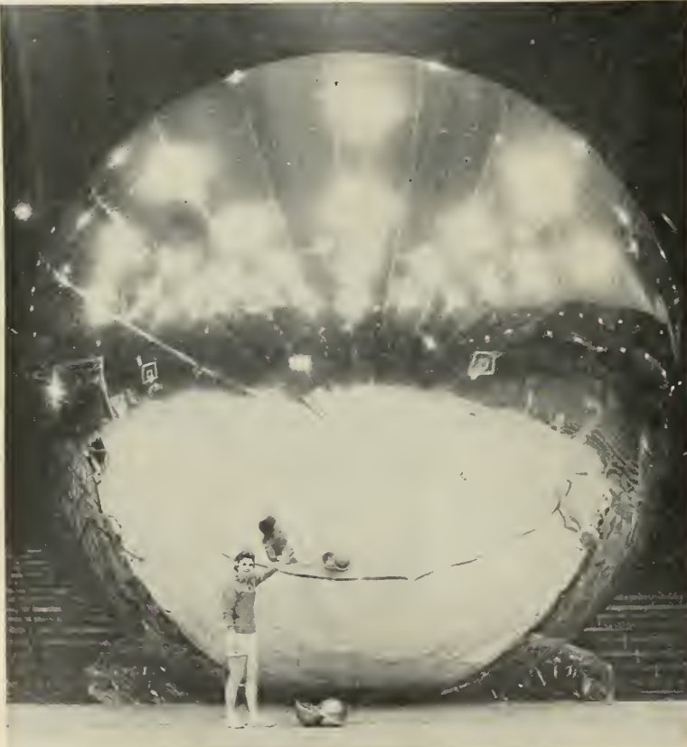
THIS 20-LB., 30'-diameter "balloonite" will be shot into a 1000-mile orbit sometime during the spring. Manufactured by G. T. Schjeldahl Co., it will carried in two small hemispheres, pictured near the young lady's feet, on a Transit vehicle.
