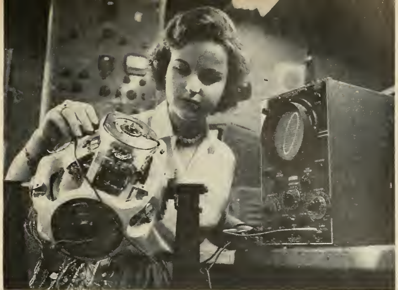
INERTIAL guidance systems—such as this model for the X-15 rocket plane shown on the “stable table”—receive exhaustive tests to determine accuracy and reliability.
