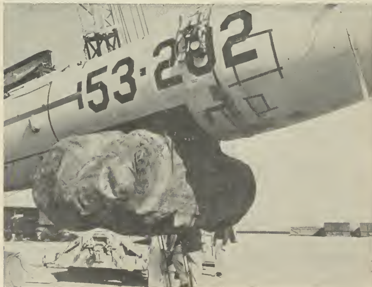
RUBBER-COATED fabric air bags fastened to the Mace missile are used as landing gear for recovery of the vehicle. Manufactured by Goodyear Tire, the recovery bags fit around the Mace's belly when popped into shape by compressed air during landing.
