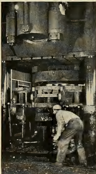
On this mammoth hydraulic press capable of exerting up to 4 million pounds of pressure, Lukens Steel Company has formed nose cone blanks for the Air Force's Atlas and Thor ballistic missiles.
