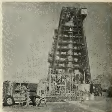
Representing the tremendous amount of ground support equipment necessary for testing ICBMs, the above photograph shows an Atlas set up for static firing of its main and vernier engines at Convair-Astronautics' Sycamore Canyon facility in California. Independent ground power units, such as Caterpillar Tractor Co.'s diesel electric generator (at left), propellant transfer facilities, and transportable vans for electronic equipment, are all big procurement subsystem items. (See Page 78.)
