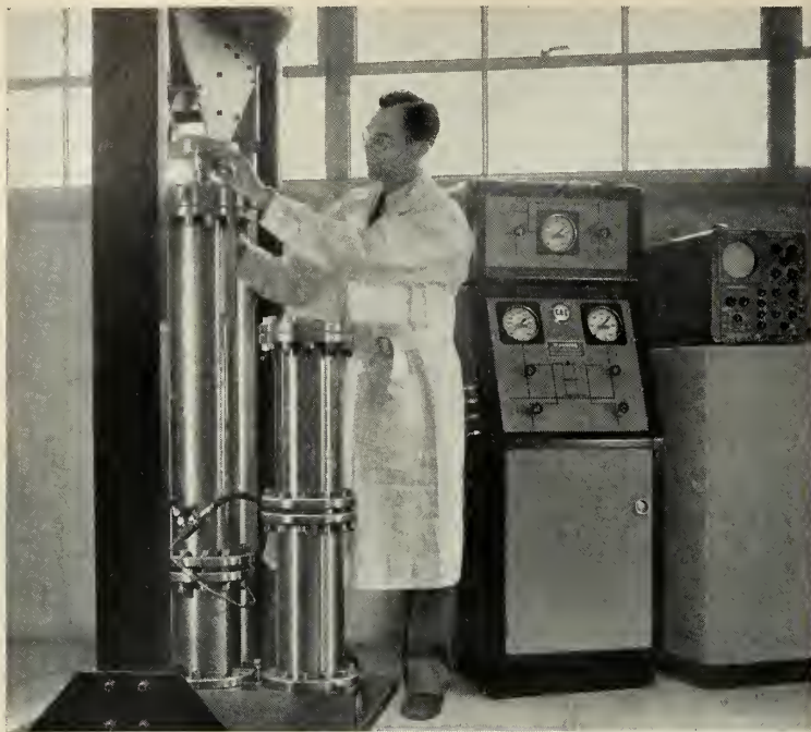
Hyge shock tester takes about 60 seconds to complete acceleration-shock test with up to 40,000 lbf. thrust. Hughes Memascope® oscilloscope retains wave pattern as long as you like for careful study and comparison with master pattern.
