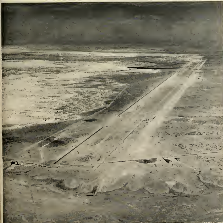
AERIAL VIEW of new 35,000 ft. rocket test track. Breech end is adjacent to track at lower left. Track headquarters are housed at right center. White sands at left.
