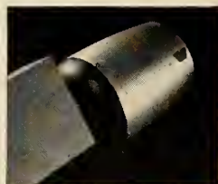
The AUTO ZOOM Lens for TV cameras using Vidicon type tubes focuses from 6 feet to infinity. Zooming and focusing can be done remotely through motorized drives.
