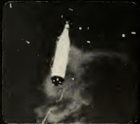
Symbolizing the Navy's future in underwater ballistic missile warfare, a Polaris FBM test vehicle erupts in a mighty geyser of water from its missile container anchored several feet below the surface of a Pacific test site. The Polaris is ejected vertically from its underwater container by compressed air in much the same manner as a torpedo. Note the four nozzles of the first stage, in the last photo.
