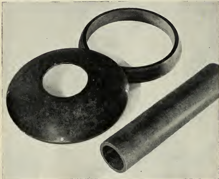
Insulator cap, blast tube and grain seat for modern rocket
