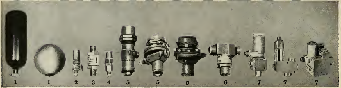
Left to right: 1 Containers (5,000 psi) 2 Relief Valve, 3 Check Valve, 4 Priority Valve, 5 Pressure Reducers, 6 Filter, 7 Solenoid Valves.
