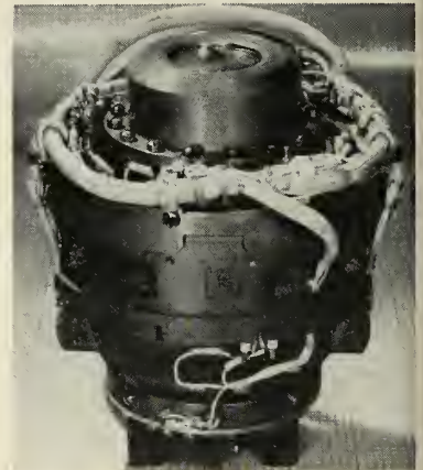
HEART of the Titan guidance system—the two-degree of freedom, torsion-wire suspended, fluid-floated gyroscope. Two gyros provide the reference system for inertial measurements.
