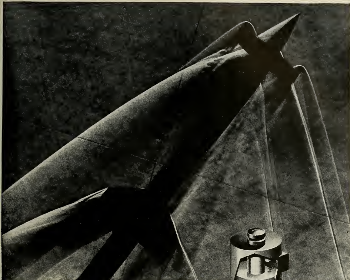
In the wind tunnel of the Naval Supersonic Laboratory at M.I.T., a missile model is subjected to speeds of several Mach numbers. B-L-H SR-4 bonded wire strain gages report longitudinal and latitudinal stresses, drag, lift, etc., with high accuracy.
