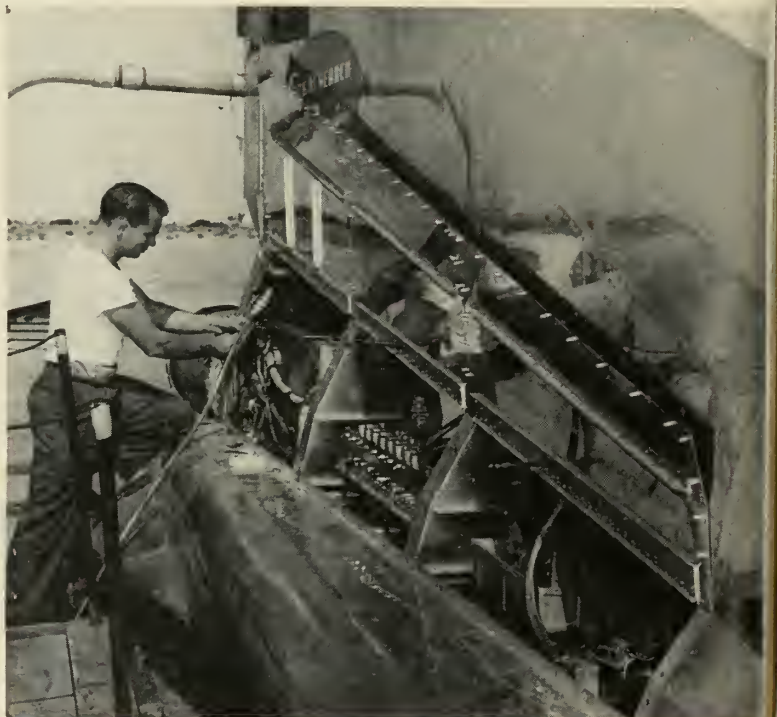
Rocketdyne engineer checks 50,000 pound thrust rocket engine used in 5000 pound Cook parachute sled. Capable of reaching 900 mph in 4.2 seconds, this unit has successfully completed 120 test runs and boasts a largely trouble-free record of performance.
