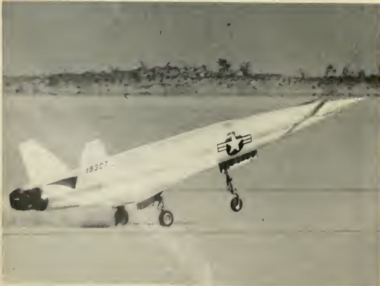
X-10 lands smoothly—coming in with nose high, easy touch-down. Note position of canard stabilizer. X-10 has been applauded by Air Force as "invaluable source of important data."
