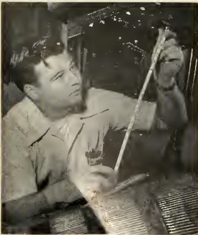
PENETRATION of solder checked by X-ray.
