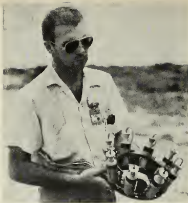
EIGHT VERNIER ROCKETS of third stage adjust its speed after separation.
