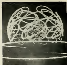
COVER: Gyration of ballistic missile flight are re-created at Avco in a three axis flight simulator.
