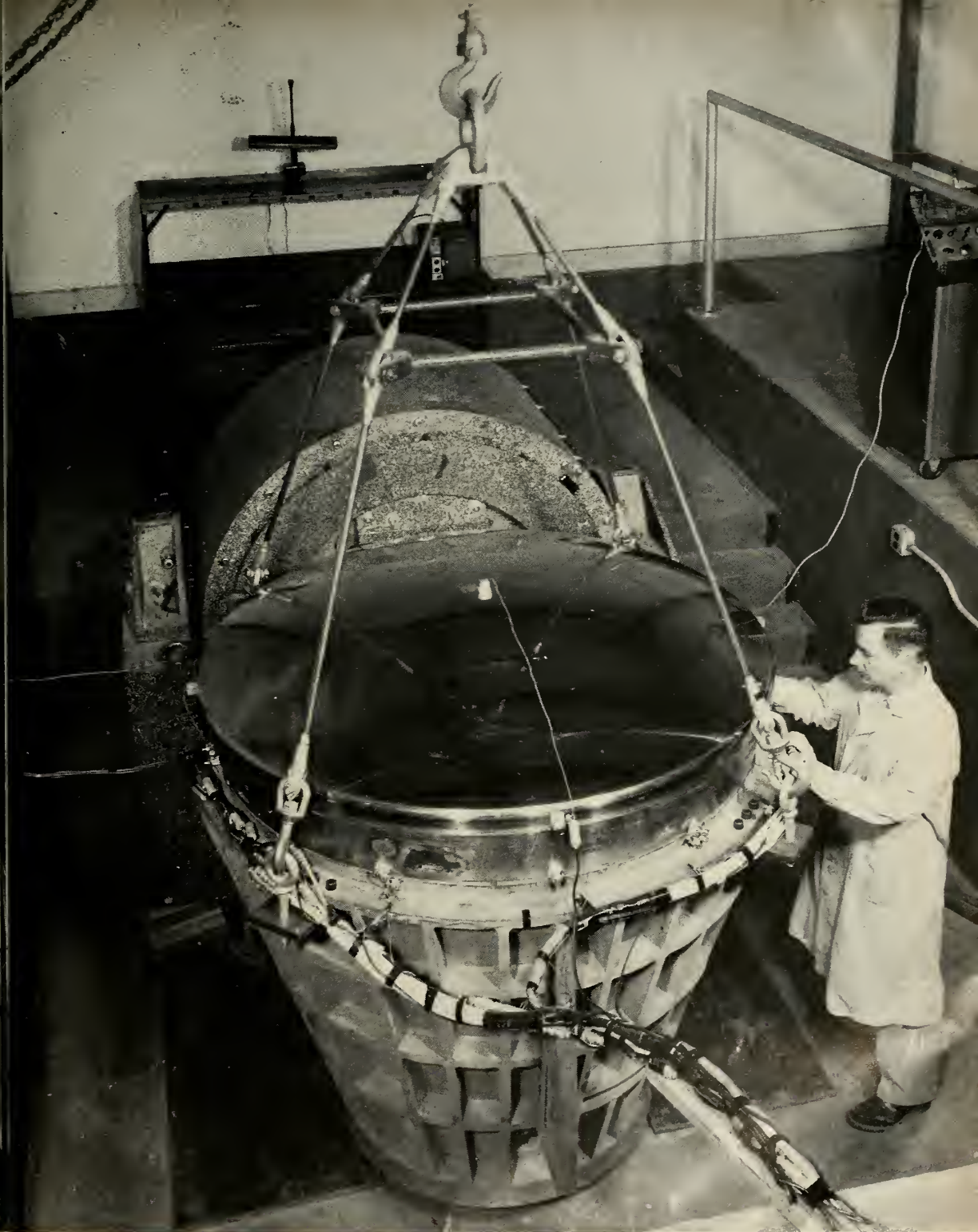
AT THE END OF THE LINE the completed vehicle receives a final vibration check before shipment to a Titan test site to make its contribution to space technology . . .
