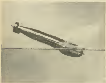
A major hydrodynamic problem with torpedoes is that they may cavitate and
