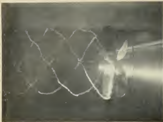
Cavitation—an equivalent of aerodynamic turbulent flow—troubles both ends of a torpedo. Fig. 1 shows propeller turbulence; Fig. 2, cavitation at the nose cone.
