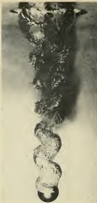
Spinning ball entering water at high speed leaves cavitation wake of water vapor similar to aerodynamic turbulent flow, exemplifying major underwater weapons system problem.
