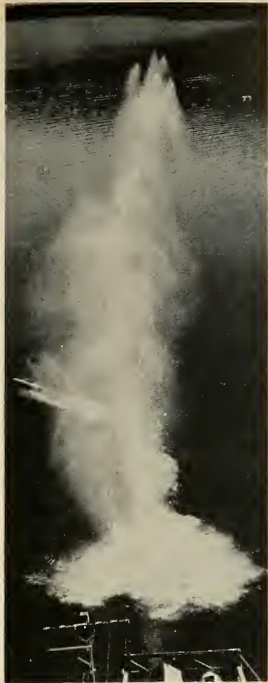
Torpedo fired to simulate aerial launch at Naval Ordnance Test Station, Inyokern, Calif., cavitates and porpoises clear of the water and almost 90° off course. This sort of thing is one of the biggest problems in underwater missile design; is a big reason why more study of the ocean and fish is needed.
