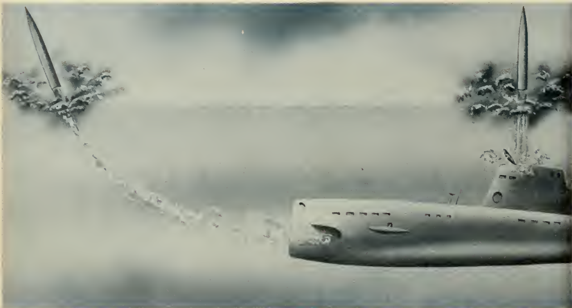
Two methods for launching underwater solid propellant rockets studied in this country are the tube-launching principle and vertical launching through the conning tower. Latter method might be employed for the Polaris . Both methods have been considered by the Russians.
