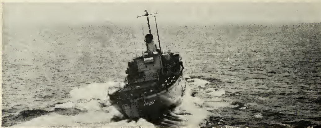
NORMALLY, STABILIZER COUNTERACTS sea movement. Here, it demonstrates effectiveness by creating man-made roll.
