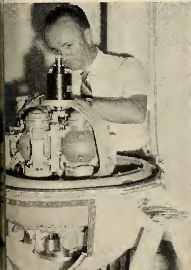
KEY ELEMENT of the ship's inertial navigation system is adjusted by engineer.
