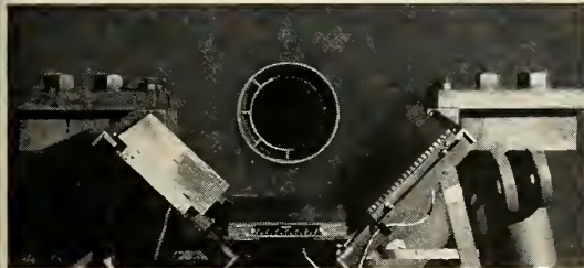
SONIC FATIGUE TESTS prove ability of Aeronca brazed honeycomb to withstand high acoustic energy levels.
