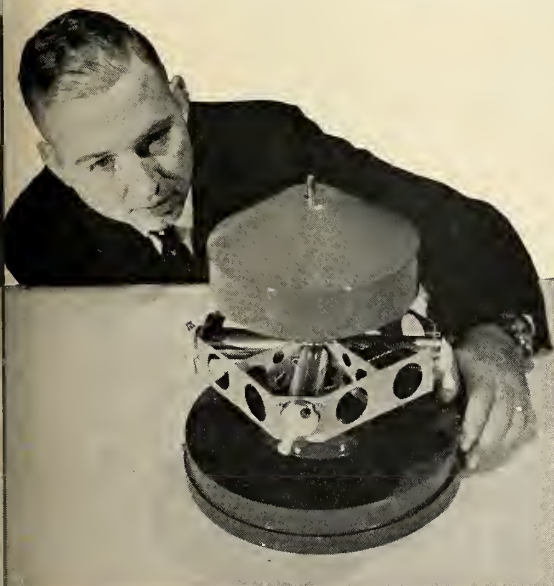
POWER STEERING for missiles is function of this set of solid-propellant attitude control rockets. A number of methods are under study at the Division's Rocket Propulsion Section.
