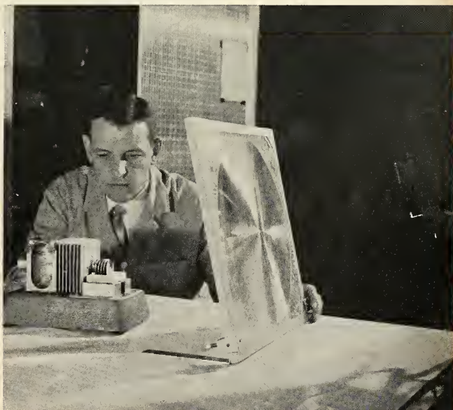
HEAT GENERATED by the arc light is collected by a Fresnel lens and concentrated on the head of a laboratory-model version of the closed cycle Stirling system.
