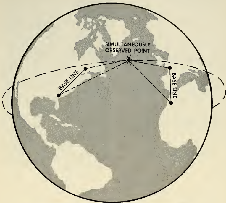
INTERVISIBLE METHOD calls for simultaneous sightings of satellite.
