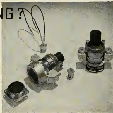
WENNER BRIDGE is used for calibrating these accurate, sealed double-wall 1-ohm standard resistors.
