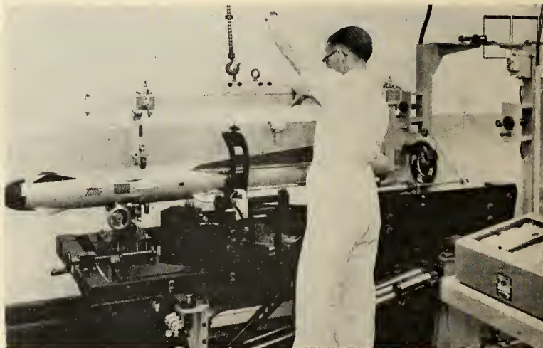
AIR HOIST guides Falcon onto platform for automatic assembly line testing.
