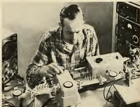
TYPICAL OF microwave equipment at the center is this X-band attenuator calibration device.
