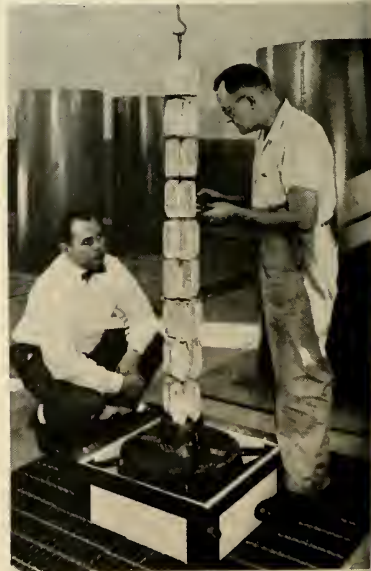
SYNTHETIC QUARTZ CRYSTALS emerge from an autoclave three weeks after the seed crystals were sealed within the vessel.
