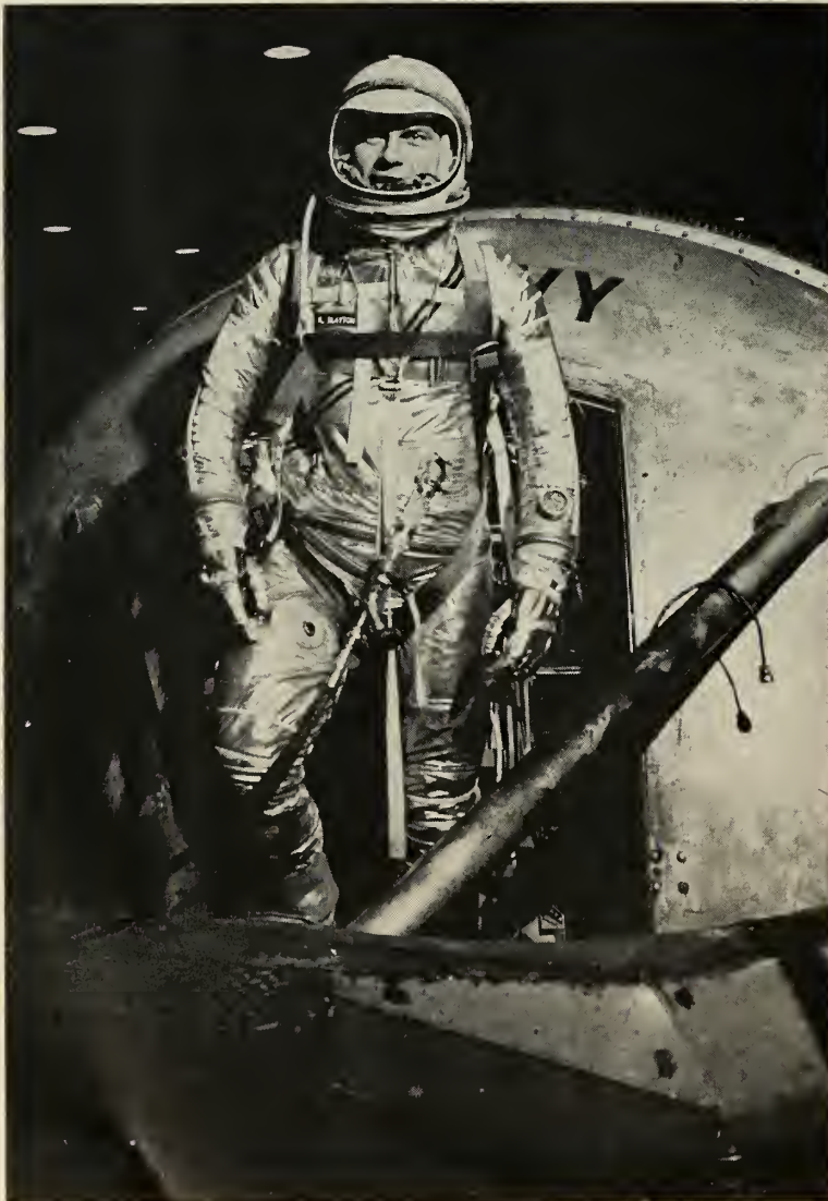
STRAPPED, VISORED AND ZIPPERED Astronaut "Deke" Slayton emerges from centrifuge chamber after a rigorous test of the new suit. In case of a cabin decompression, the orbiting astronaut could not live more than 10 seconds without the suit.
