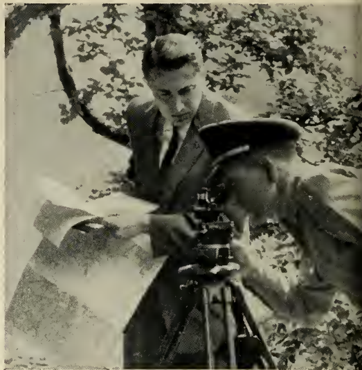
In Germany, checking a proposed radar site for masking objects, preparatory to installation.
