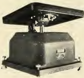
Model 1411—Roll-Pitch-Yaw Test Table 0° to 15° from horizontal, 6 cycles per minute (standard), automatic reversing of direction of motion can be set from one to twelve cycles; table motion symmetrical. For testing all Gyro-Directional instruments, and limbering up runs on Gyro-Horizon indicators and for Automatic Pilot Control units. $345.00
