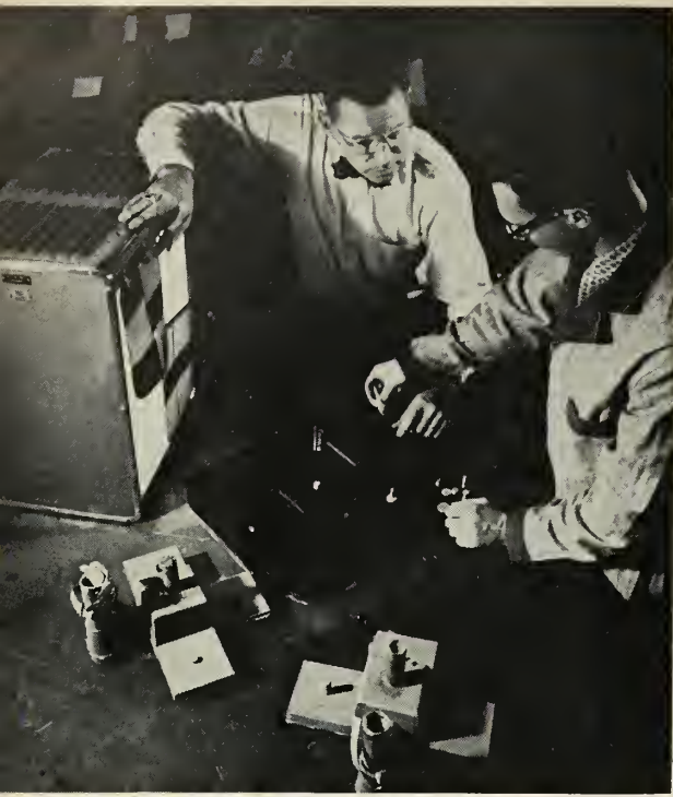
FLAWS ARE DESIGNED into the castings by the tiny silver discs which the engineer is here arranging on the pattern board.
