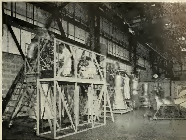
ROCKET ENGINE Fitting Bay where Rolls Royce LOX/kerosene engines are assembled for the Blue Streak.
