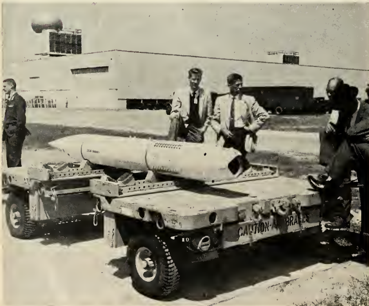
MHU-12 TRANSPORT TRAILER carries four Bullpups at speeds up to 20 mph. Adjustable chocks and available sideboards make the unit a multipurpose vehicle.
