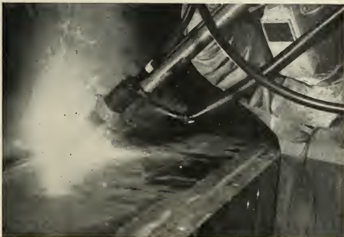
Machine welding heavy aluminum armor plate in FMC's Ordnance Division's shops.
