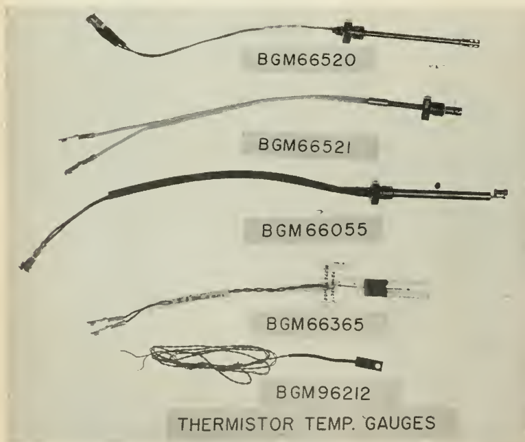
Above is an array of typical thermistor temperature gauges for measuring inflight conditions during test firing of the REDSTONE.
