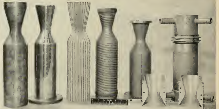
Chambers left to right: Spun, finished, corrugated, hydraulically or cast formed, chamber with flow directors braced on and outer casing suitable for any type rocket chamber. Further information is available by contacting NACA and requesting NACA Technical Note 3827.
