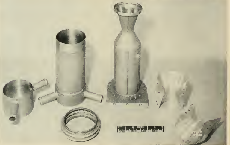
Spun chamber with outer channels for fuel flow control. Left, casing. Right, throat.
