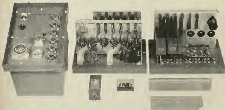
How the REDSTONE minds its measurements. Above is a typical signal adapter for converting inflight measurements into telemetry signals. Shown in the picture are the various plugs for gauge input, power supply inputs, outputs to go to the telemetering system and the large plug for pre-flight check-out service. These components can be spotted about the missile as space is available.
