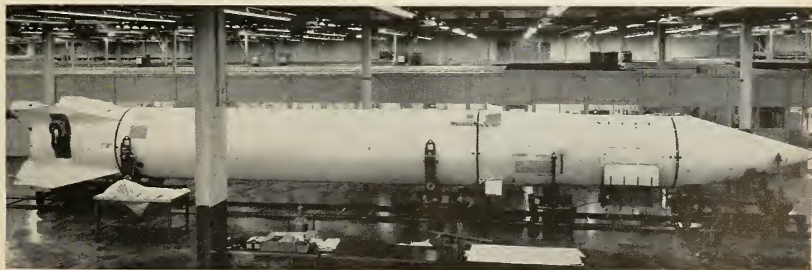
A production ballistic missile, REDSTONE is being weaponized for issue to field forces.
