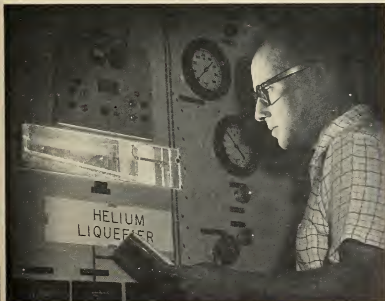
LIQUID HELIUM being produced in the laboratory. This NBS Boulder Lab Engineering Research Tool is capable of putting out about 5 gal. of liquid helium per hour.
