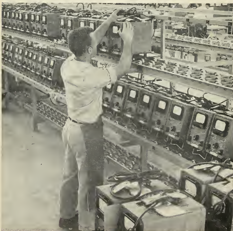
HEWLETT-PACKARD is representative of electronics activity in the Bay area, employs 2000. Here new voltmeters are assembled for testing at HP's Stanford plant.
