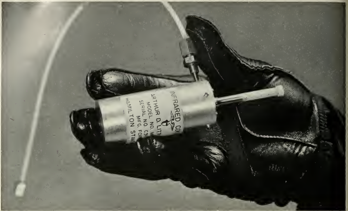
MinIRcooler developed by ADL. Available from Hamilton Standard for IR applications. High altitude glove by David Clark Co., Inc., courtesy of U. S. Air Force.
