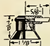
≅90 or 91SCCOSL beryllium copper contact, cadmium plated nests in anti-corona cup. Skirt clings to tube—guards against flash-over. Silicone rubber insulation throughout.
