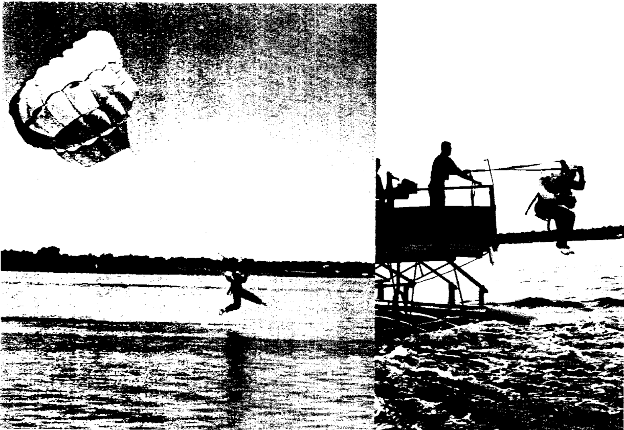
WATER WALKER —A drop in the wind velocity causes a parasail to be sluggish in lifting off as the pilot seemingly runs across the surface of Lake Texoma. At right, pilots jump from the stern of a moving barge with parachute risers attached to simulate being dragged by an inflated parachute after a water landing.
