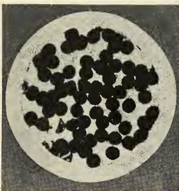
ALTERNATE form of the wire consists of multiple Pd and Al wires in an Al jacket.
