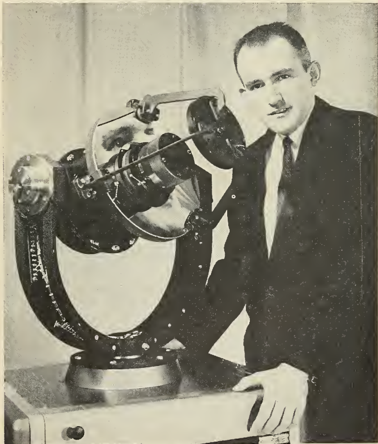
FAR INFRARED Gyroscopic Scanner is demonstrated by Irving E. Distelhorst, project engineer at Martin's Baltimore Division. The 50-lb. unit was displayed publicly for the first time at the recent IRE convention in New York. The gimbal support ring, mounted on a controls console, can rotate 360° on its vertical axis; the scanner and mirrors assembly can rotate 360° on a separate horizontal axis.
