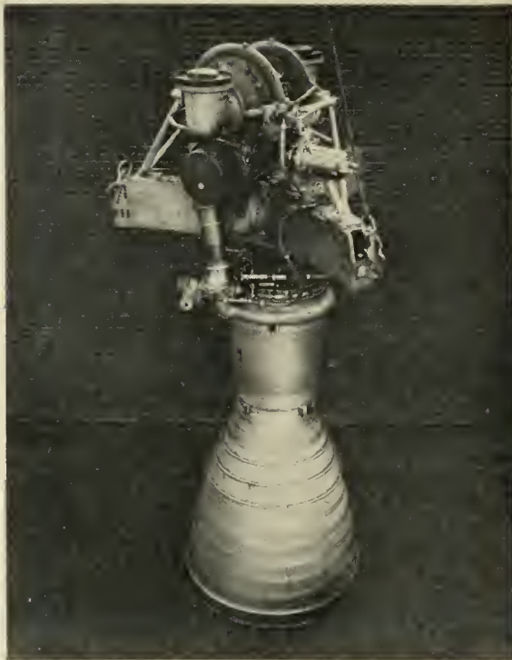
X-1 ENGINE uses beam-type mount rather than usual tripod type to save weight, reduce fabrication time. Solid propellant turbine spinner is in dome at upper right.
