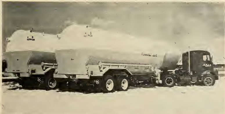
TWO HYDROGEN TRAILERS built by Air Products await delivery to Air Force.
