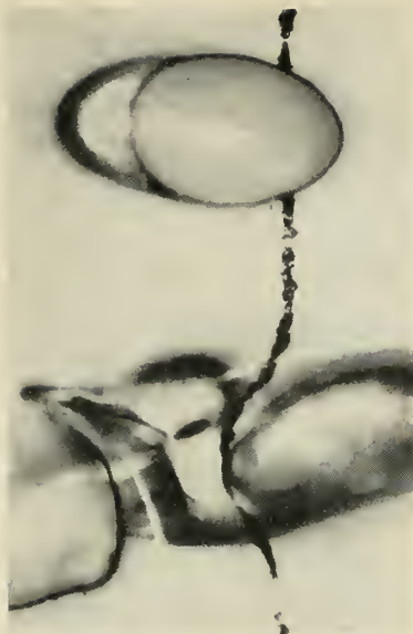
GAS bubbles, resulting from repeated stressing on the surface of an aluminum specimen, appear under a strip of transparent tape. The horizontal line is powdered metal extruded from the fatigue crack.
