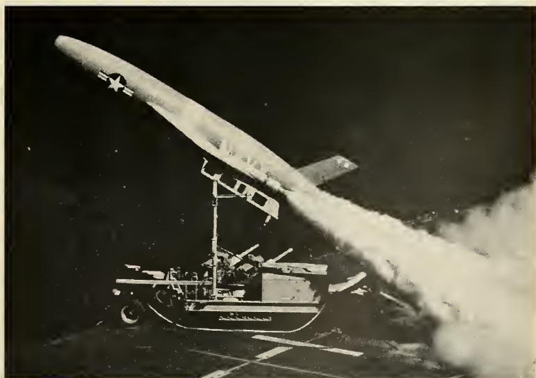
A ZERO-LENGTH launch is made from deck of carrier, boosted by rocket power.
