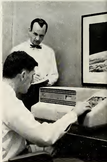
Prototype model of ASI Digital System Simulator is designed to give direct check of reduction of logic equations, to study a system's operations prior to construction, and to study alternate logical designs.
