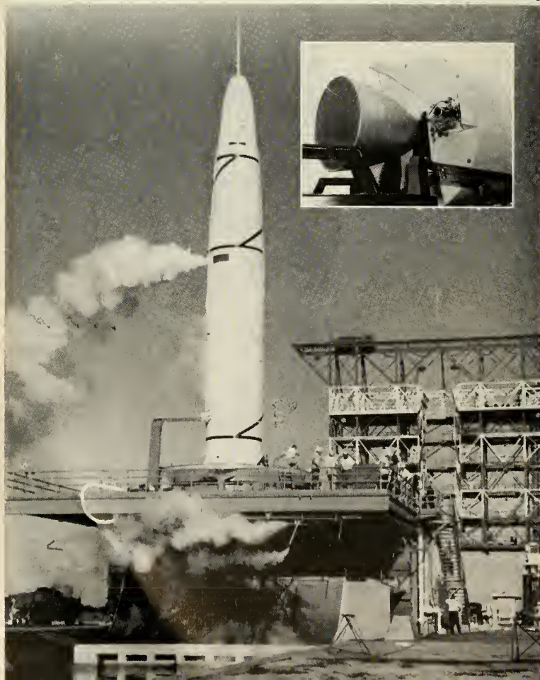
LIQUID OXYGEN is "topped off" as Thor is prepared for test flight from the Cape. USAF; (Inset) Howard Levy
