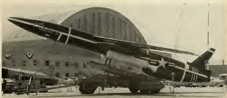
SNARK CAN BE quickly readied for action with its mobile transport-launcher.
