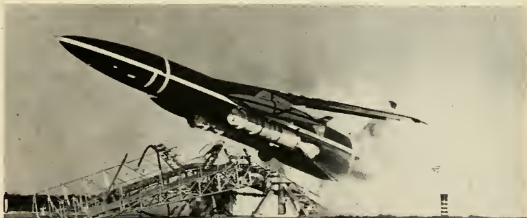
THE 25-TON Snark clears its zero-length launcher with a 66,000-lb. assist.
