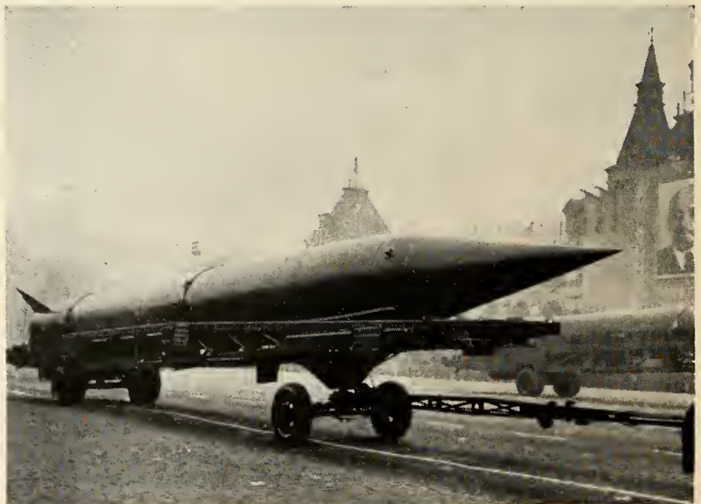
THE SOVIET T-1, AN IMPROVED GERMAN V-2, mainstay of the SSM program.
