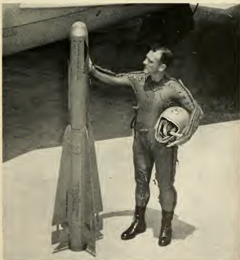
THE PSEUDO-CANARD Falcon GAR-2A is equipped with infra-red detection system.
