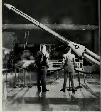
Far Side Missile developed by Aeronutronic for Office of Scientific Research. Four-stage rocket was balloon launched and fired to record high altitudes where they measured the Earth's magnetic field and cosmic radiation intensities.
