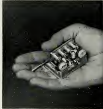
ASI Model IL-101 Subminiature Transmitter provides exceptional frequency stability under high acceleration space conditions. Size of unit: 1.1 x 1.4 x 2.1 inches. Weight: less than 5 ounces. Output: 150 ± 5 mW.
