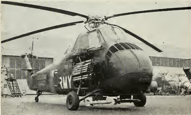
PRESENTLY UNDERGOING TESTING is the Sikorsky H-34A. Armament includes forty 2.75 inch rockets, two 5-inch rockets, two 20-mm cannon, and six machine guns.
