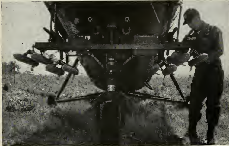
VERTOL H-21C mounting 80 mm Oerlikon rockets and .30 caliber machine guns. Tests were conducted at the Army Aviation School, Fort Rucker, Alabama.
