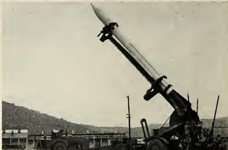
Army THE CORPORAL is positioned on its pad by a LeTourneau transport-erector.
