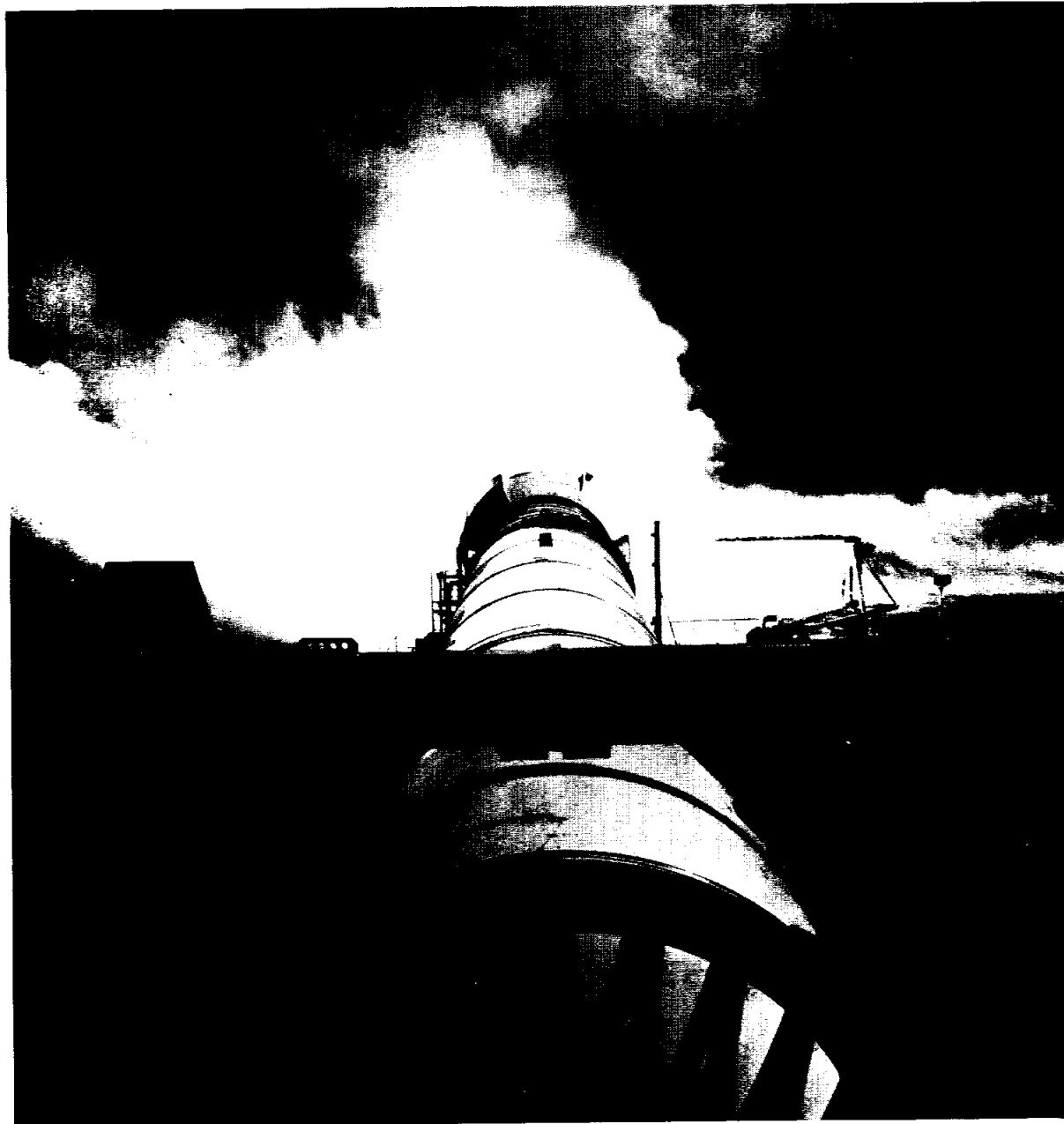
Development Motor 8 roared to life Aug. 30 in the first full-scale, full-duration firing of the new solid rocket motor design. The next firing is scheduled for November.
