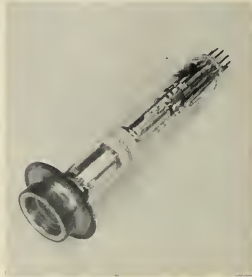
THERMICON thermal imaging tube being developed by Westinghouse for track-while-scan, multiple target handling.
