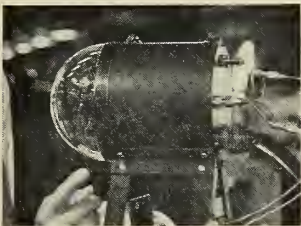
SIX-INCH diameter scanning head is a recent development in infrared airborne intercept equipment. A survey of the complex but promising IR market starts on p. 25.
