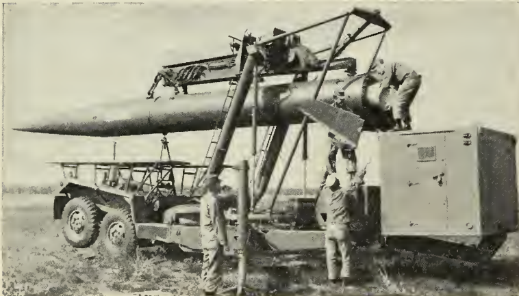
MINUTES IS ALL it takes to assemble Sergeant on its mobile launcher. Sergeant vehicles mark first use of U.S. Steel's newly developed thin sections of T-1 steel.
