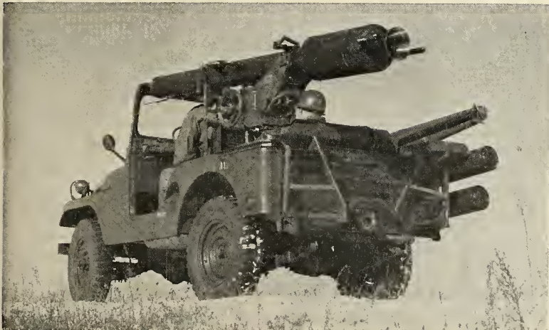
ARMY UNVEILS Davy Crockett mortar-launched tactical missile with nuclear or HE warhead. New defense bill calls for production of more than 6000 of this new missile.
