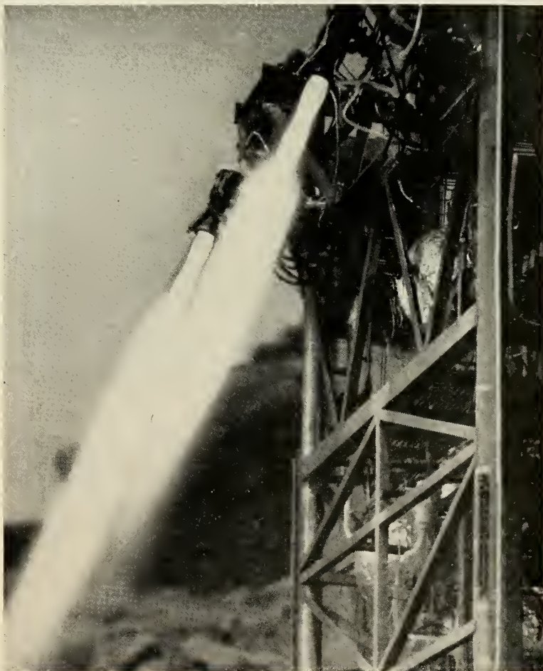
ATLAS VERNIER engines generate 1000 lbs. thrust for 1930 seconds at Rocketdyne's Propulsion Laboratory, Canoga Park, Calif., in the longest run ever made by a rocket engine. Hydromatics Inc., Livingston, N.J., manufactures Flo Ball valves, which control LOX and fuel flow. Hydromatics says its valves are used on all major liquid rocket projects, including Thor , Titan , Jupiter , X-15 , Nova and Centaur .
