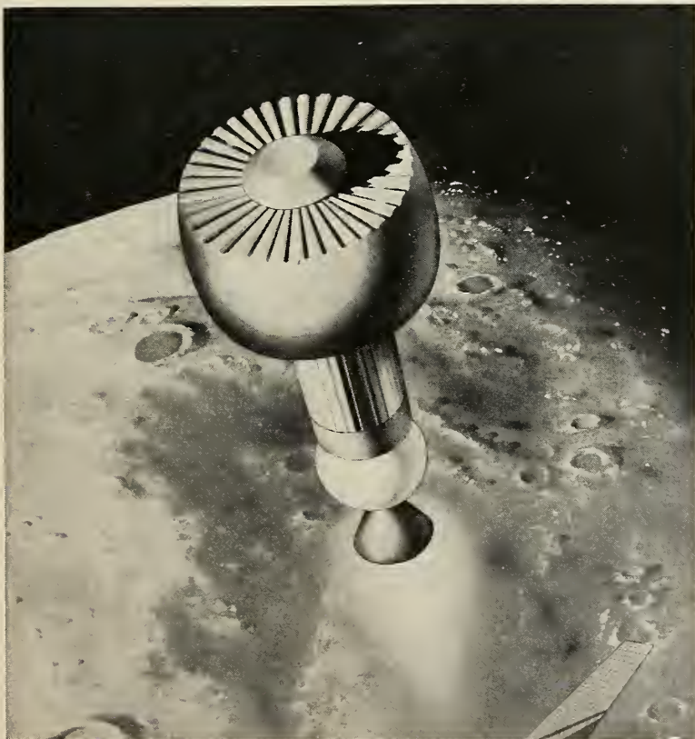
MOON LANDING attempt by NASA within two years will use 300-lb. instrumented capsule developed by Ford's Aeronautic Division. Retro-rockets will lower capsule from 20 miles out. Drawing shows capsule after separation from vehicle.
