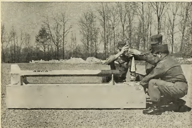
ROCKET-BORNE radioonde, developed by Army Signal Research and Development Laboratory and produced for the Signal Corps by Atlantic Research Corp., is loaded into nose cone of ARCAS rocket. It will separate 40 miles up and float down.
