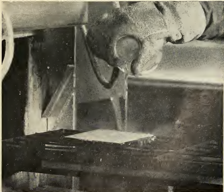
THERMAL SHOCK of 1200 FΔT, caused by pouring ice water on a Nucerite plate at 1250°F, resulted in no visible damage to the ceramic coating.
