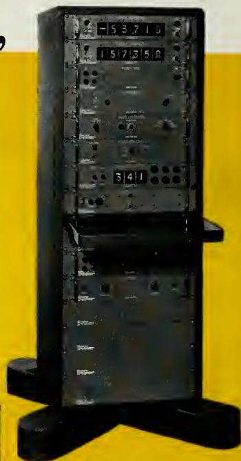
Multi-purpose digital system for measuring a variety of transistor parameters while the transistors are being subjected to environmental testing.
