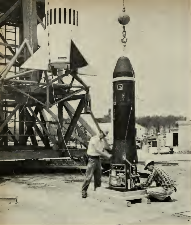
ALTAIR fourth stage of NASA's Scout is given last-minute checks at Wallops before being raised to its final position atop the first three stages of the space exploration vehicle.
