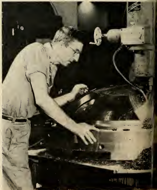
SECOND-STAGE FORWARD CLOSURE is checked for thickness at Allison. The fixture adjacent to the dome stabilizes closure configurations during heat treat
