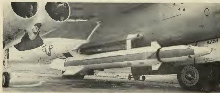
MARTIN BUILT 199B ALBM shown attached to B-47, manned by a Martin Company crew, which took off near Baltimore Oct. 13 and fired the two-stage Air Force R&D bird into the vicinity of paddlewheel satellite Explorer VI over Atlantic Missile Range near Cape Canaveral.
