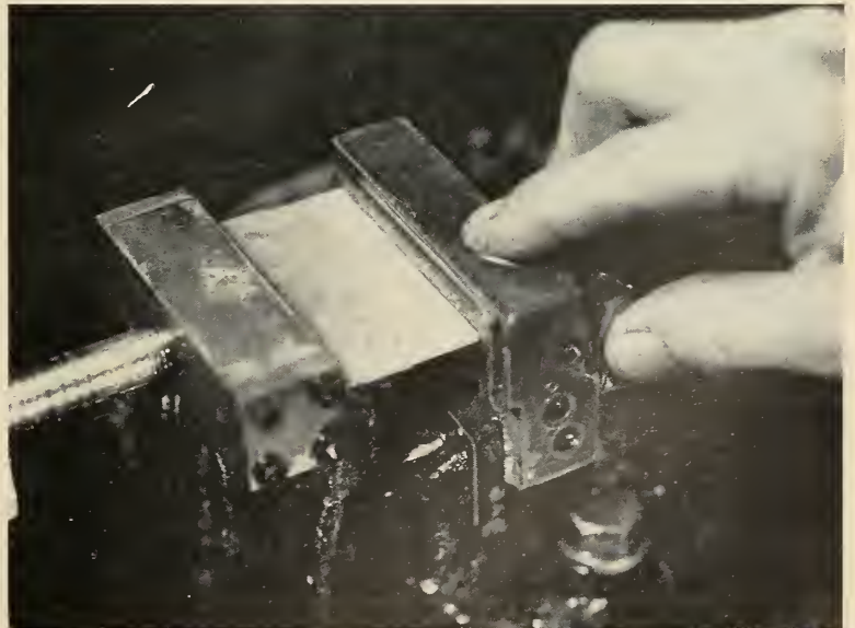
ANOCUT'S electrolytic cavity-sinking machine forming a narrow slot with a knife-type electrode. Note that low heat permits operator to keep fingers on workpiece.
