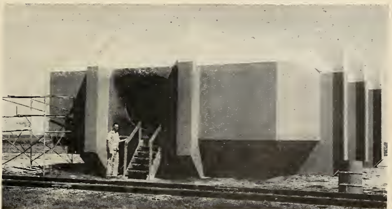
SIMULATED shipboard missile magazine is used for damage evaluation tests of bulkheads, venting, sprinkler and drainage systems and for stowage safety tests.
