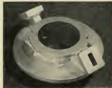
THIS SAND CAST WAVE GUIDE was held to \pm .005 " on passageway dimensions. Surface smoothness requirements are 63 RMS. The foundry has government approval for any phases of its operations where such approvals are applicable.
