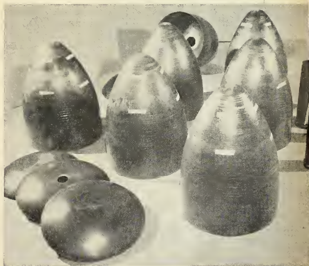
COMPLETED ASSEMBLIES contain the dome-shaped bulkheads for concentricity stabilization and stiffness.
