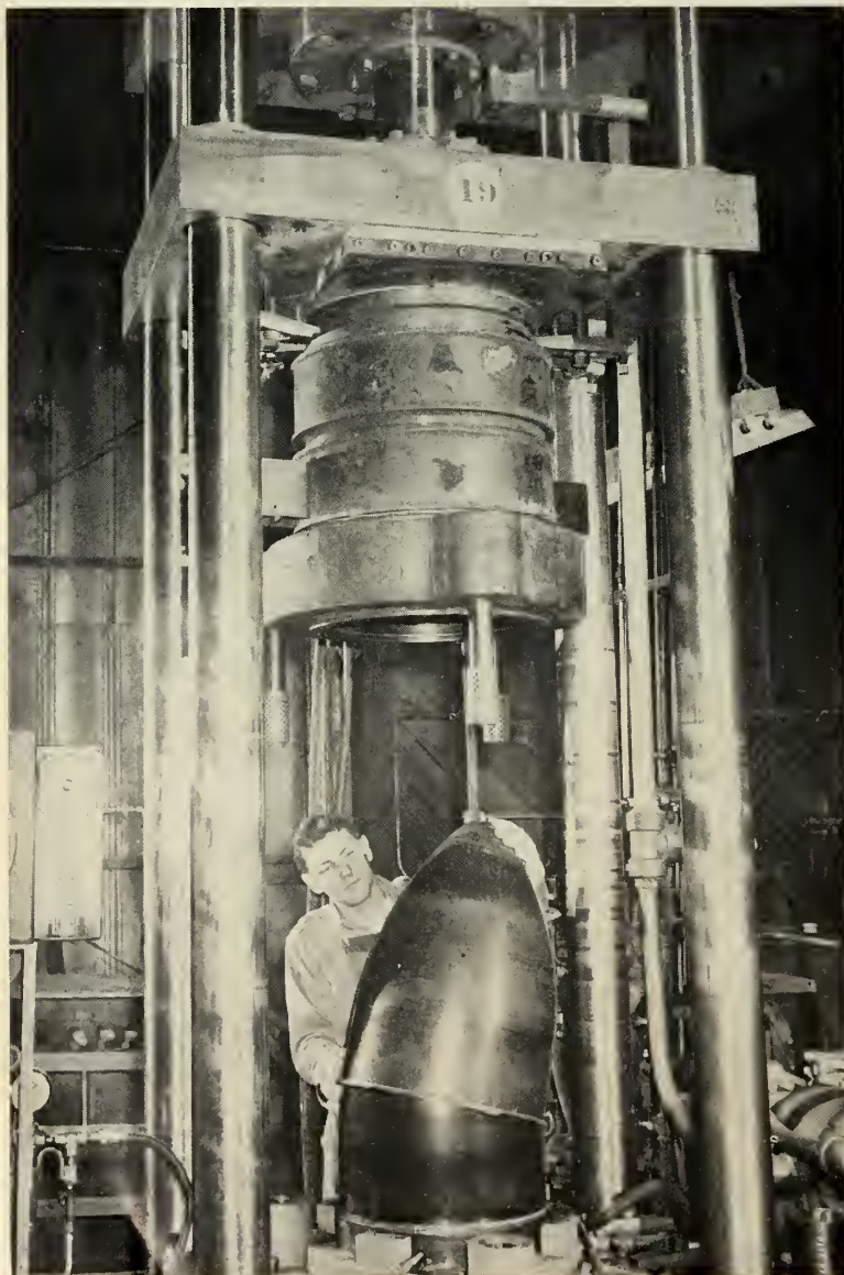
POLARIS NOSE FAIRING is compression-molded to net dimensions with matched metal tooling in heated, high-pressure equipment.
