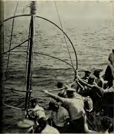
ANTENNA FOR detecting electromagnetic fields is lowered for calibration tests.
