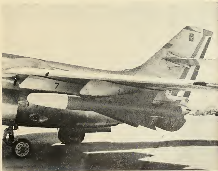
MATRA R. 530, here mounted on Vautour, has electromagnetic and infrared guidance.
