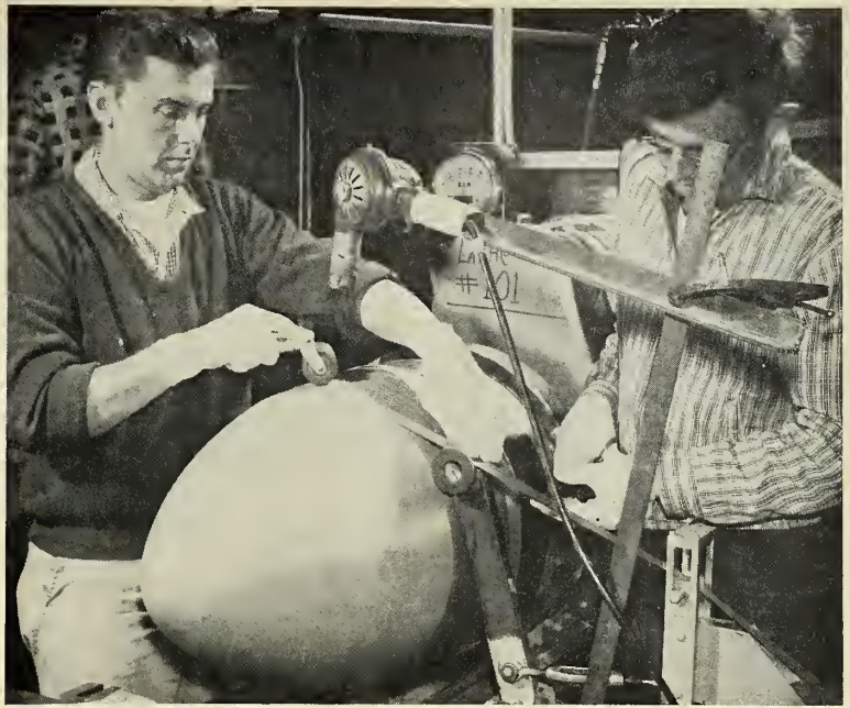
OUTER SHELL is wound shingle fashion with overlapping layers of tape. The inner shell visible is composed of seven layers of glass cloth.
