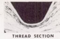
FIGURE 13. SILICIDE COATED COLUMBIUM ALLOY BOLT
