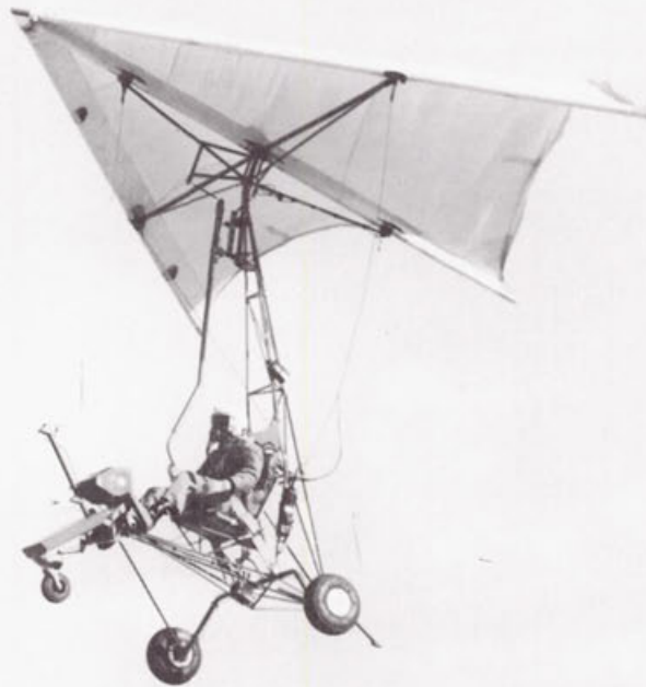
Figure 11. - Paraglider research vehicle built and flown at NASA Flight Research Center, Edwards, Calif.
