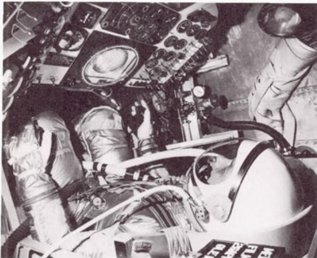
FIGURE 2. Mercury Astronaut in AMAL centrifuge gondola during training and simulation in preparation for Mercury Redstone and Mercury Atlas space flights.
