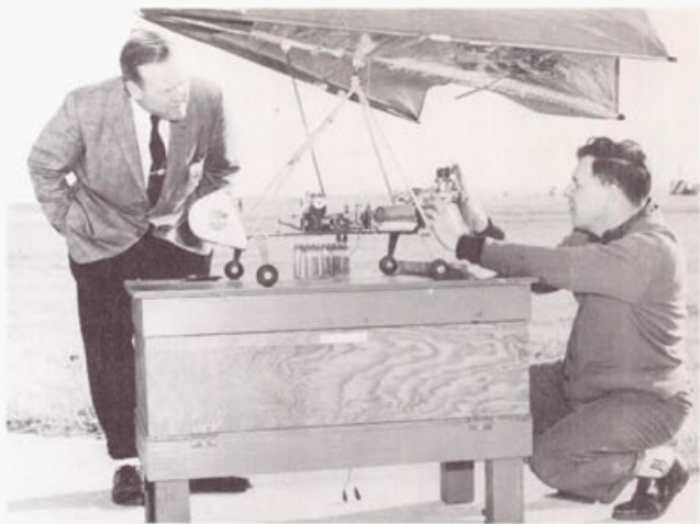
Figure 7. - Radio-controlled gas-powered model of a manned flexible-wing vehicle being prepared for flight by the Langley Recovery Systems Branch.
