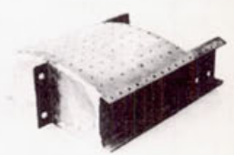
FIGURE 5. PROTECTIVELY COATED MOLYBDENUM ALLOY ASSEMBLY STRUCTURALLY TESTED AT 2500°F.
