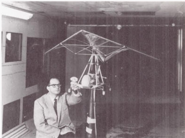
Figure 8. - Static wind-tunnel model of a manned flexible-wing vehicle in a Langley 7- by 10-foot tunnel.
