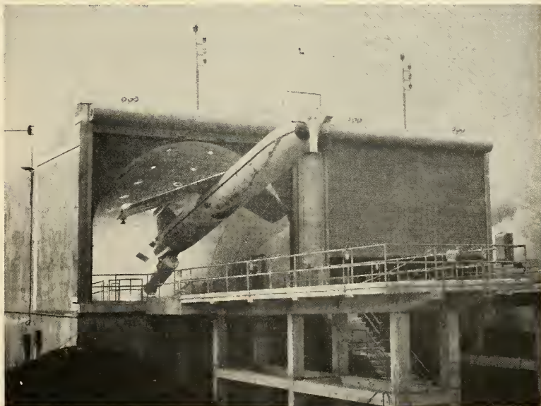
PROTOTYPE OF MACE B hardened launcher was proved out in a July 11 shot at Cape. Sites will be used in West Germany. The Martin tactical missile was kept on "hot hold" for several hours before firing.
