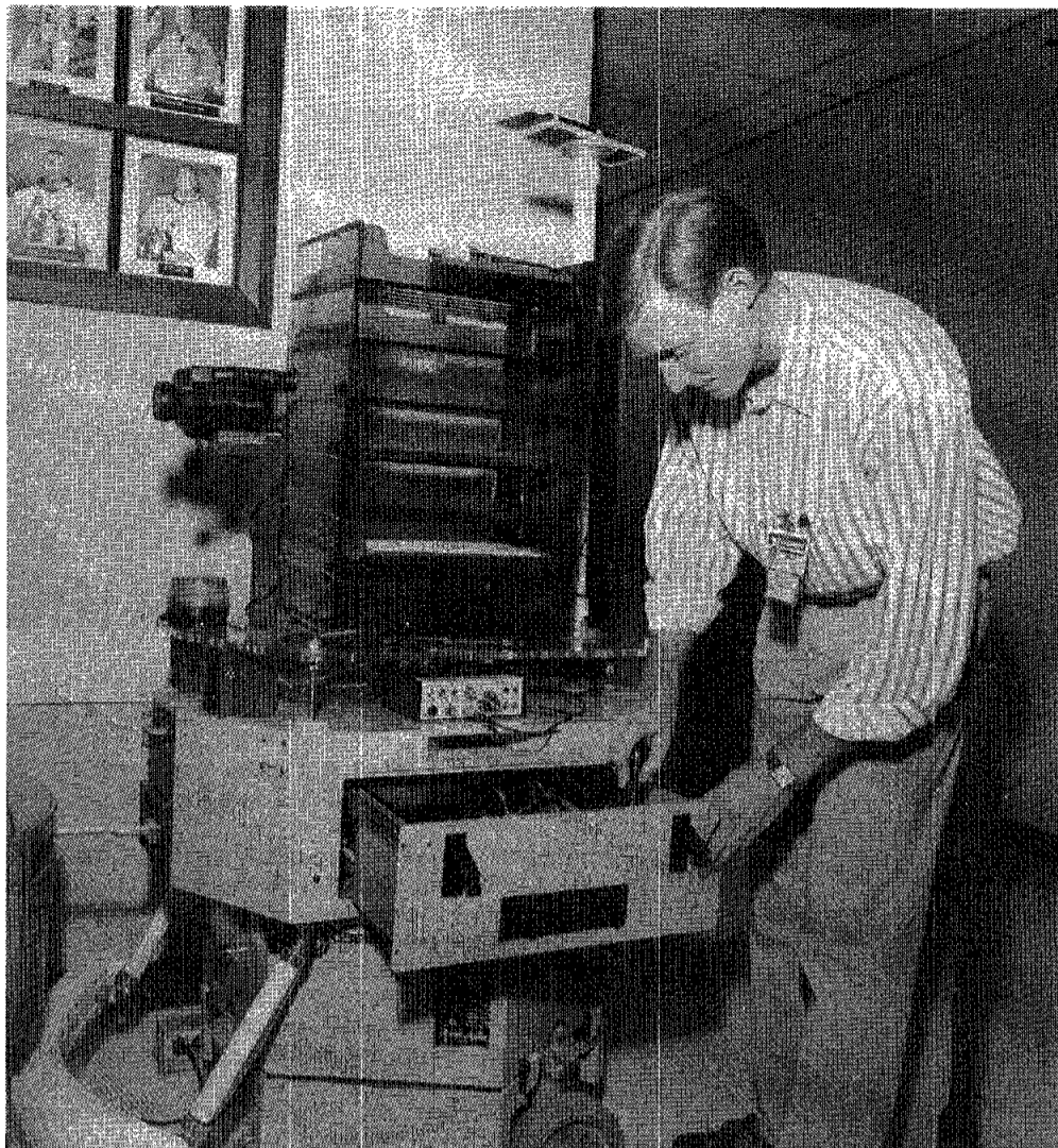
Above: Lockheed robotics engineer Bill Cravers makes an adjustment to "Jasper" between mail runs. Cravers assists Project Engineer Don Rhoades with fine-tuning the robot's software. Jasper delivers mail to six branch offices seven times a day, and, in a year of service, has proven extremely reliable. Right: Sharon Williams, secretary for the Robotics Systems Technology Branch in Bldg. 32, loads mail into the Mail Delivery Robot. Below: Rhoades works on the personal computer in his office that is used to track and command the robotic mailman. A television monitor displays the view from a camera mounted on the robot, and a map of the building on the computer displays its current location. Bottom: Connie Alexander, a counselor who heads the Employee Assistance Program on the first floor of Bldg. 32 and is blind, can tell where the robot is by listening for music from its stereo and a chime clock. She's affectionately named her mechanical coworker "Jasper."
