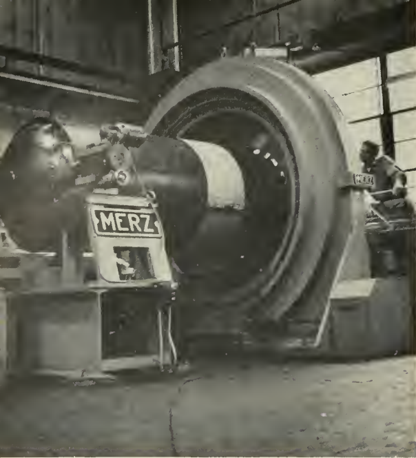
← THREADING operation being performed on a motor case. Note the sheer bulk of the machining tool necessary to insure that the threads have the required precision.
