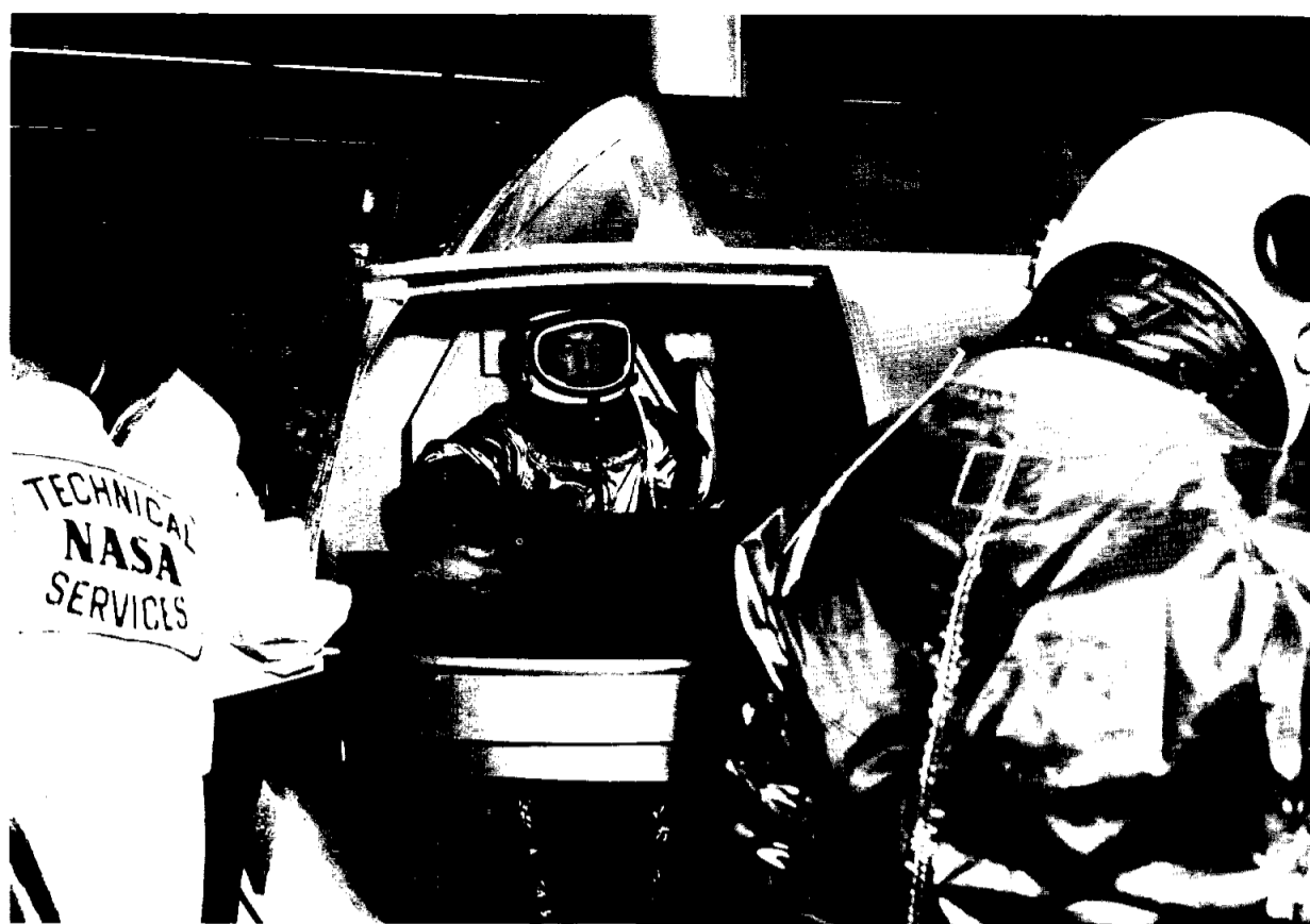
A PLYWOOD MODEL of the lunar excursion module, full scale, was constructed in MSC's Technical Services shop recently for demonstrations during contract negotiations with Grumman Aircraft Engineering Corp. Astronaut Scott Carpenter here demonstrates how pilots would fit in.
