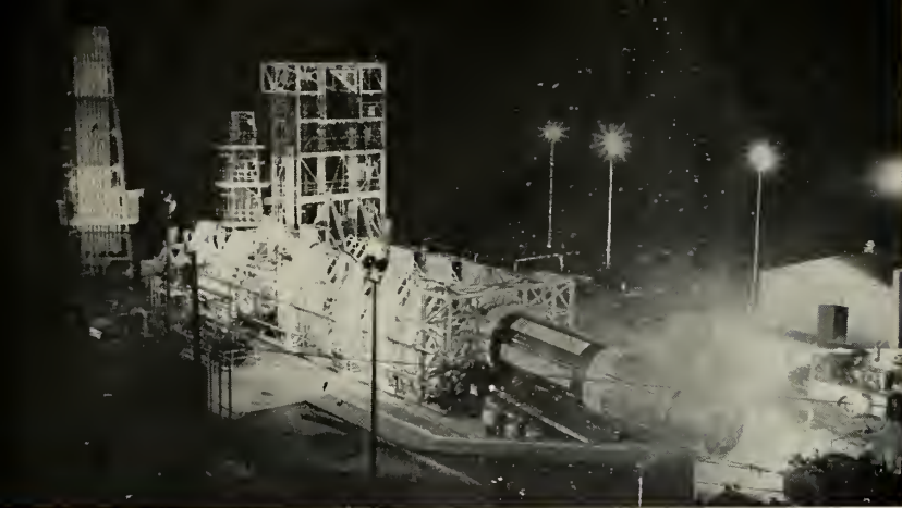
TITAN'S FIRST STAGE is removed from the erector following a static firing at the Denver Division of The Martin Co.
