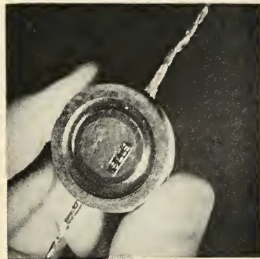
ONE-WATT vacuum thermionic converter produced by General Electric's Power Tube Department will be commercially available next month. The close-spaced sealed-off unit has minimum power density of 0.2 watts per square centimeter of cathode surface and thermal efficiency of at least 2.5%.
