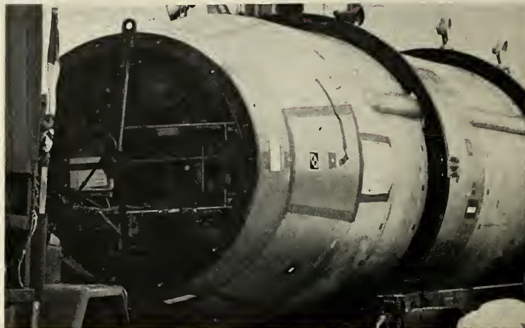
TITAN I COMMAND GUIDANCE instrumentation, in upper section of 2nd stage, just aft of warhead, includes radar beacon, autopilot, command receiver and decoder.
