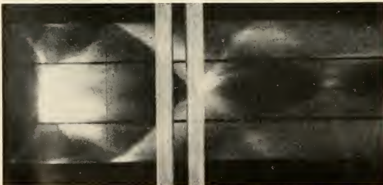
STREAK PHOTOGRAPH of cylindrical pinch was taken through 0.05 slit in upper electrode.
