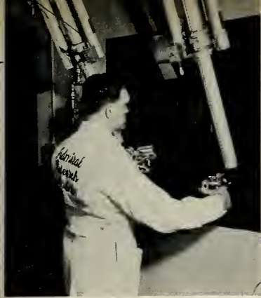
ADMIRAL CORP. nuclear engineer remotely handles components in the company's 20 kilocurie cobalt 60 radiation chamber.
