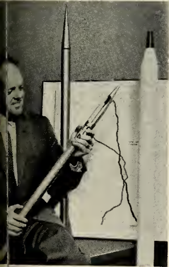
ELECTRONICS , Borg-Warner Corp. has developed the Owl meteorological probe for ARDC to provide wind direction and velocity information at altitudes as high as 240,000 ft.
