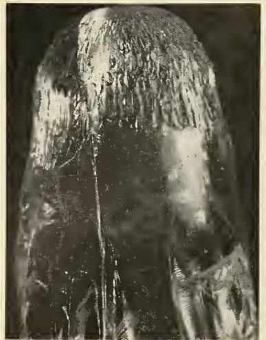
ABLATED QUARTZ model. Up to 100% pure silica has been tested successfully, but shielding value drops in re-entry.
