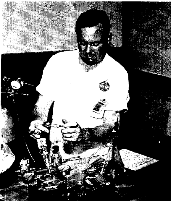
DAN CARTER JR., equipment specialist, Crew Systems Division, Environmental Control System Laboratory, prepares for a centrifugal water separator test.
