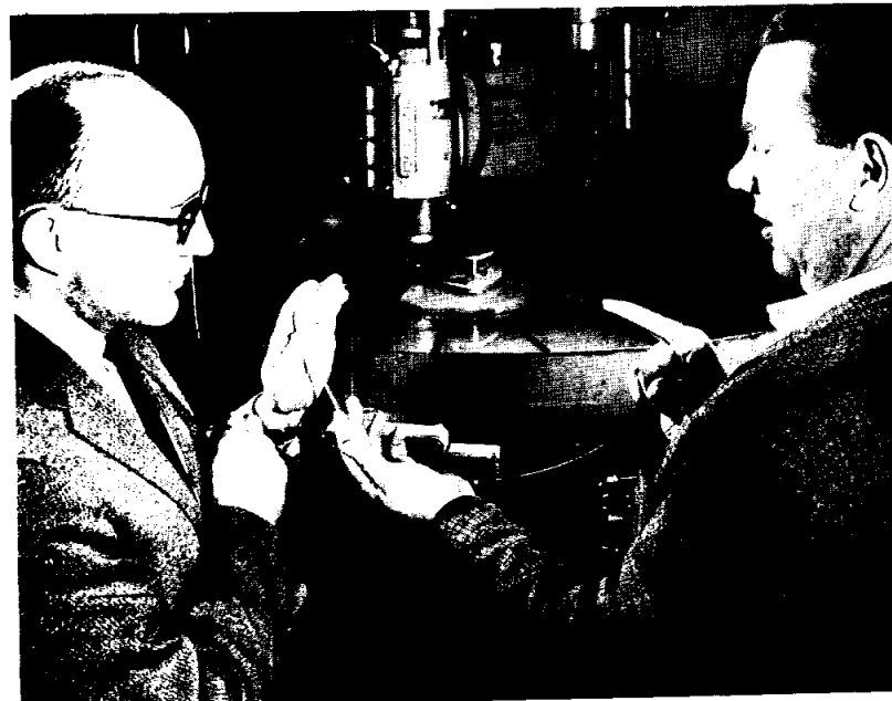
GEMINI WINDOW --Each of the eye-shaped windows on the Gemini spacecraft consists of three panels like this one. Size of the window is about eight by 17 inches. The outer panel is resistant to high temperatures, the inner panel is specially strengthened to resist mechanical shock, and the middle panel performs both functions.
