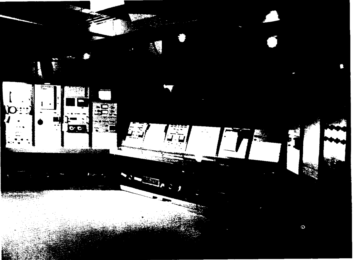
MASTER CONTROL CONSOLE for the transfer locks within the Vacuum Laboratory are shown on the second floor of the LRL. Scientists will monitor the transfer of the samples from one area to another via this master console.
