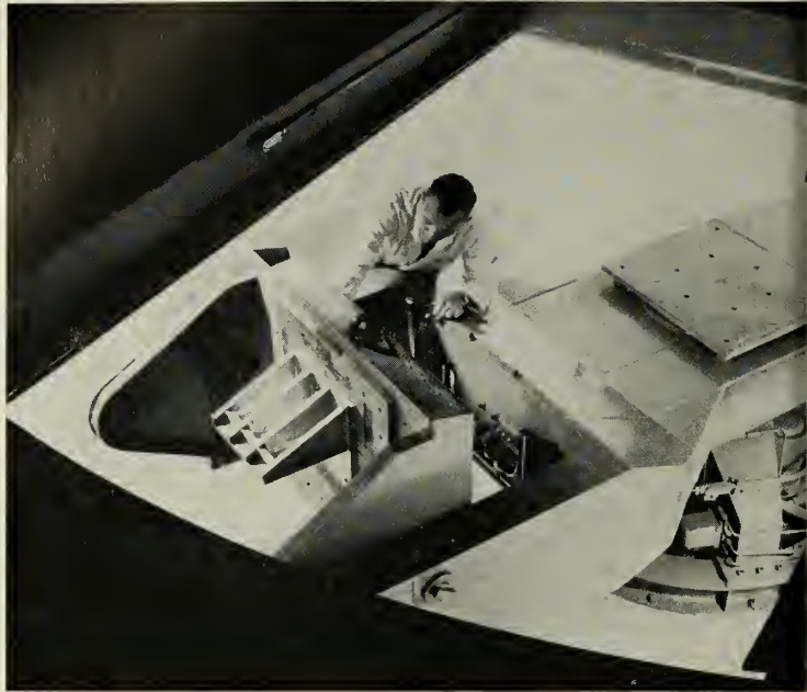
(below right) Large centrifuge for environmental testing has unique shaker attachment to provide vibration simultaneously with high G-loadings.
