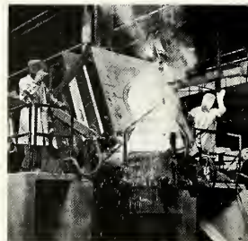
5,000-lb. heat of special alloys is produced from this unique melting furnace.
