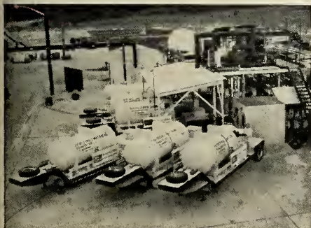
25,000 POUNDS OF LIQUID FLUORINE, from General's Metropolis, Ill., Works — ready for over-the-highway shipment in tank trucks of our own design to rocket and missile research centers throughout the nation.
