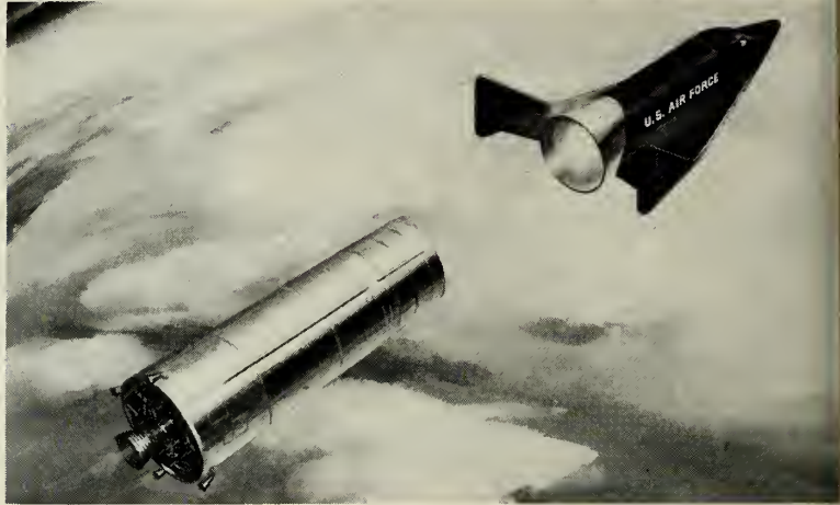
SECOND-STAGE Titan booster falls away in artists conception, leaving Dyna-Soar in piloted, near-orbital flight.
