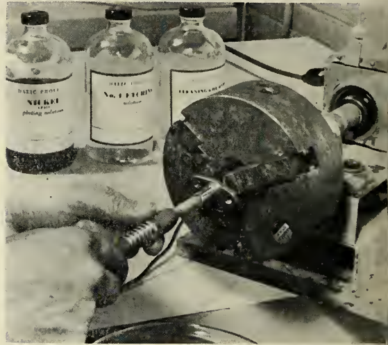
FUEL INJECTION nozzle for turbine after-burner receives 0.0004 to 0.0006-in. plating of nickel on inner diameter and chamfer.
