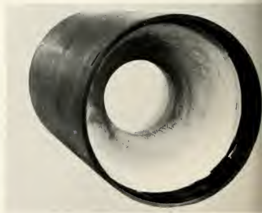
The ceramic material in this 10" O.D., 11" long rocket nozzle was designed to operate in the exhaust of a high energy aluminized fuel solid propellant rocket.
