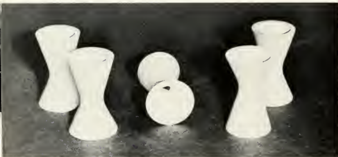
Westinghouse formed these ceramic rocket nozzles for test firing in a MERM (materials evaluation rocket motor).
