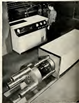
This Model 1200 Dynapak is capable of delivering 160,000 ft. lbs. of energy.
