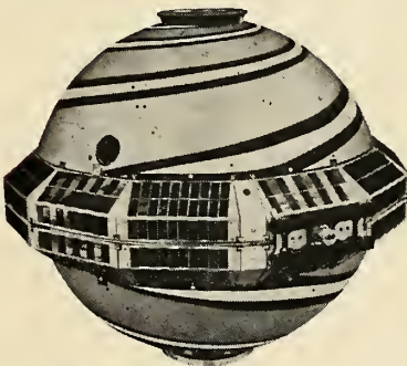
R&D TRANSIT has band of solar cells and painted spiral antennas (white lines). In smaller operational model, most of surface will be solar cells, different type of antennas will be used.
