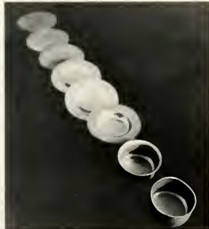
Cup-forming sequence as shown by interrupted samples.
