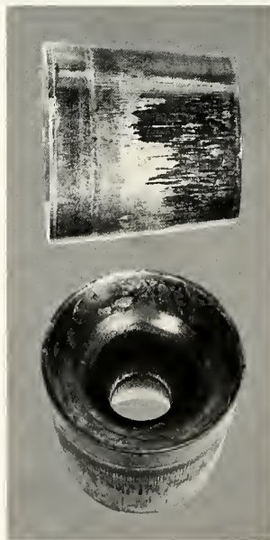
A high temperature and a high deformation rate was used to make this pure tungsten nozzle on the Dynapak.
