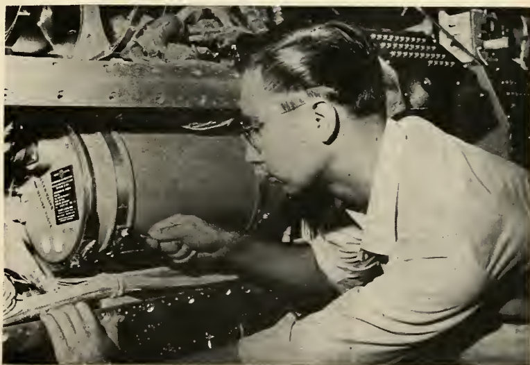
ELECTRIC Silvercel battery by Yardney is being installed in an Air Force ICBM, to supply main power during flight. It discharges 300 amps at 26 volts for 10 minutes.
