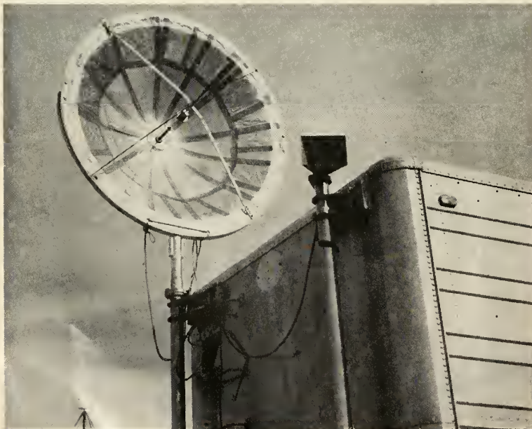
RADAR ANTENNA was built from discarded nose cone shipping cover partially filled with plastic and covered with aluminum foil.
