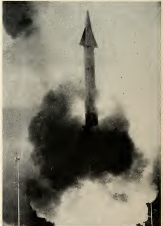
SECOND CONFIGURATION of Zeus , with most fins removed, was launched from underground silo at White Sands April 28.
