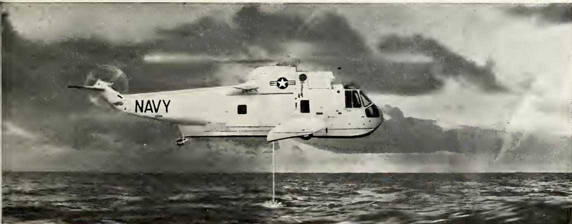
SIKORSKY HSS-2, designed for long over-water flight and low-altitude hovering—even alighting on water—during sanar anti-submarine missions.
