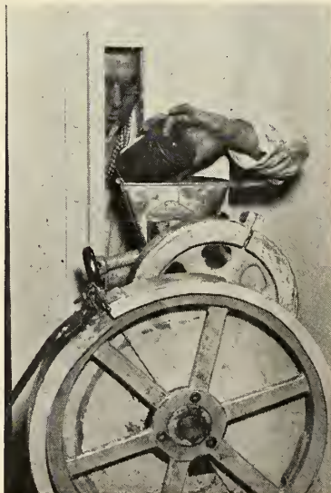
PROTECTED behind heavy glass and steel partition, worker pours propellant ingredient into mixing bay hopper.
