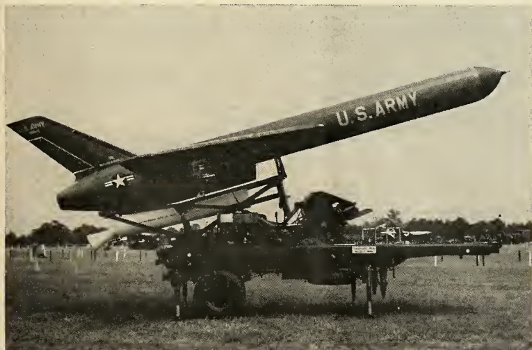
FIRST PICTURE of Army Signal Corps' AN/USD-5, Fairchild Engine and Airplane's surveillance drone, shows bird on its mobile ground launcher.
